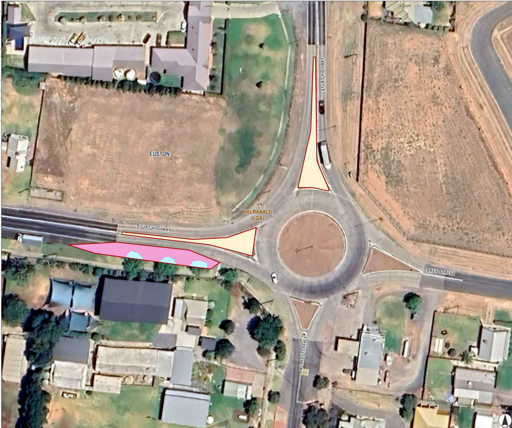
FIGURE 4.9 Features of Off-site Road Works - Euston
