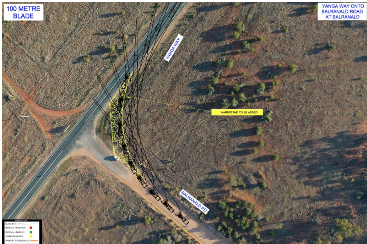
Figure 2-3 Proposed design for works at the intersection of Yanga Way onto Balranald-Moulamein Road (Rex J Andrews 2024).
