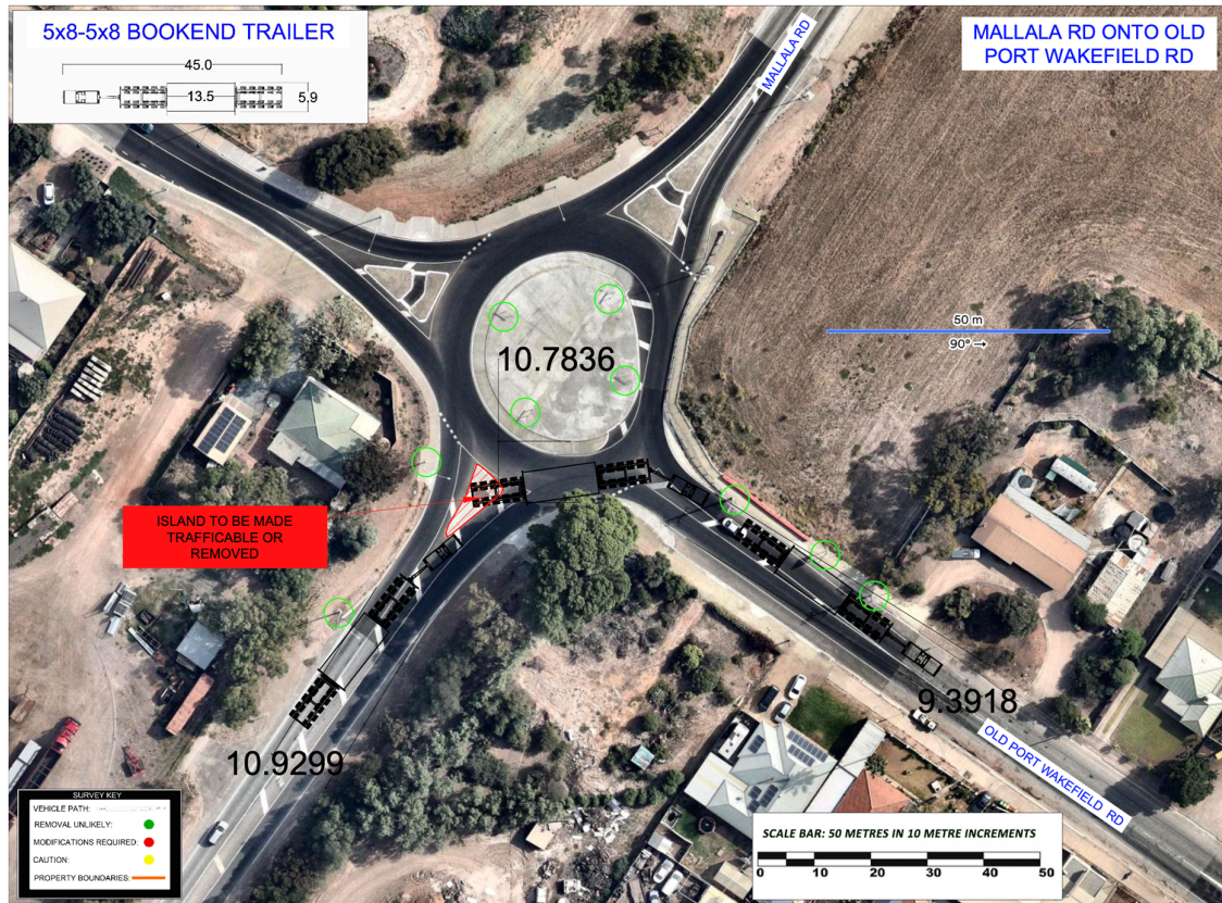
Figure 40 – Mallala Road onto Old Port Wakefield Road
