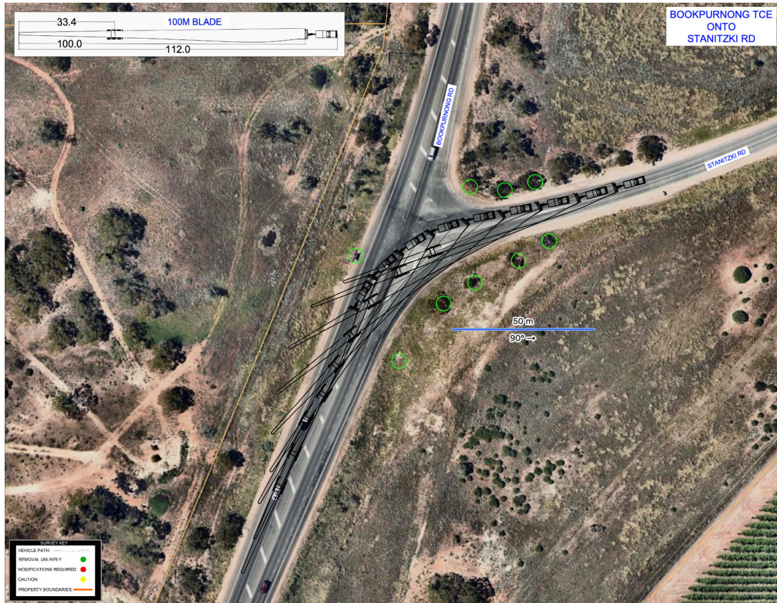
Figure 11 - Bookpurnong Road onto Stanitzki Road, SA.
