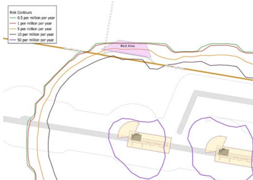
Figure 3 LSIR Contours After Relocation of WTG 177
