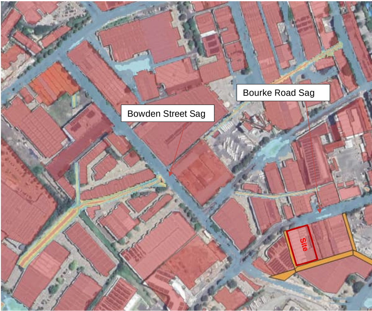
Figure 10 10% AEP flood hazard plot showing Bowden Street trafficable, and the centre of Bourke Road trafficable
