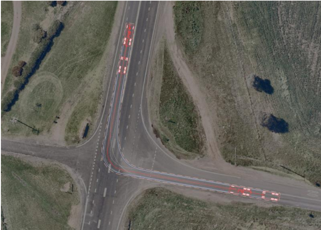
Figure 4-6: 19 m truck-and-dog right turn swept path from Burrendong Way into Mitchell Highway
