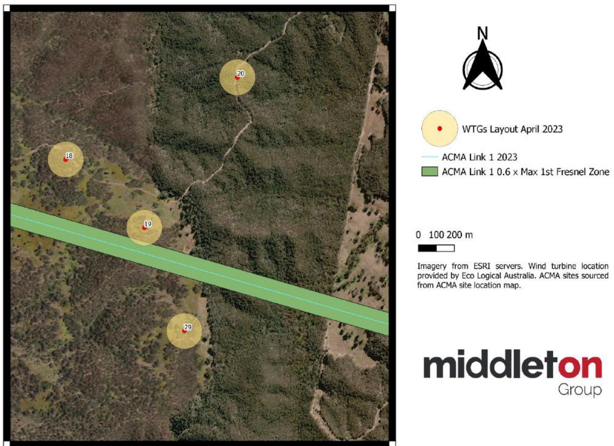
Figure 4-7: WTG 19 envelope based on 180 m rotor diameter, relative to 0.6 multiplied by maximum 1st Fresnel Zone extent of Link 1 (Middleton Group 2024b)
