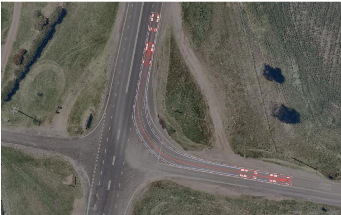
Figure 4-5: 19 m truck-and-dog left turn swept path into Burrendong Way from Mitchell Highway
