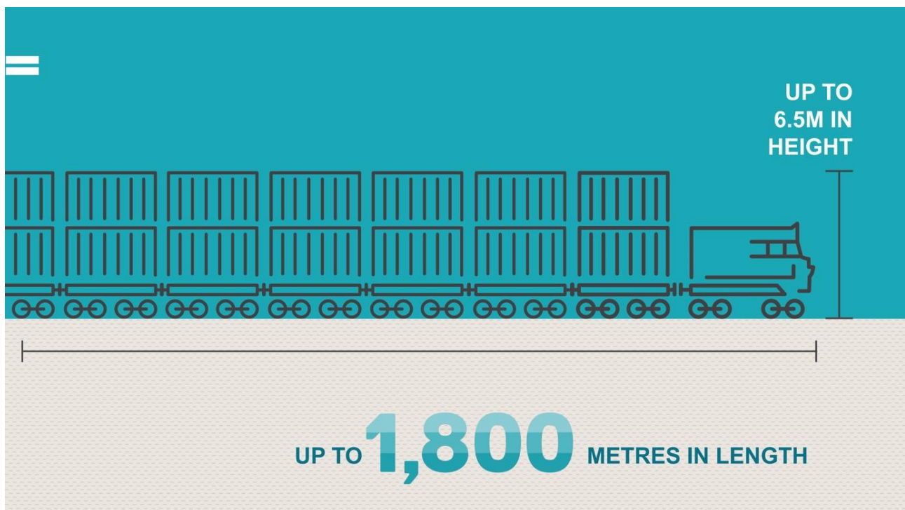
FIGURE 1-3: INDICATIVE HEIGHT AND LENGTH OF A DOUBLE-STACKED INLAND RAIL FREIGHT TRAIN
