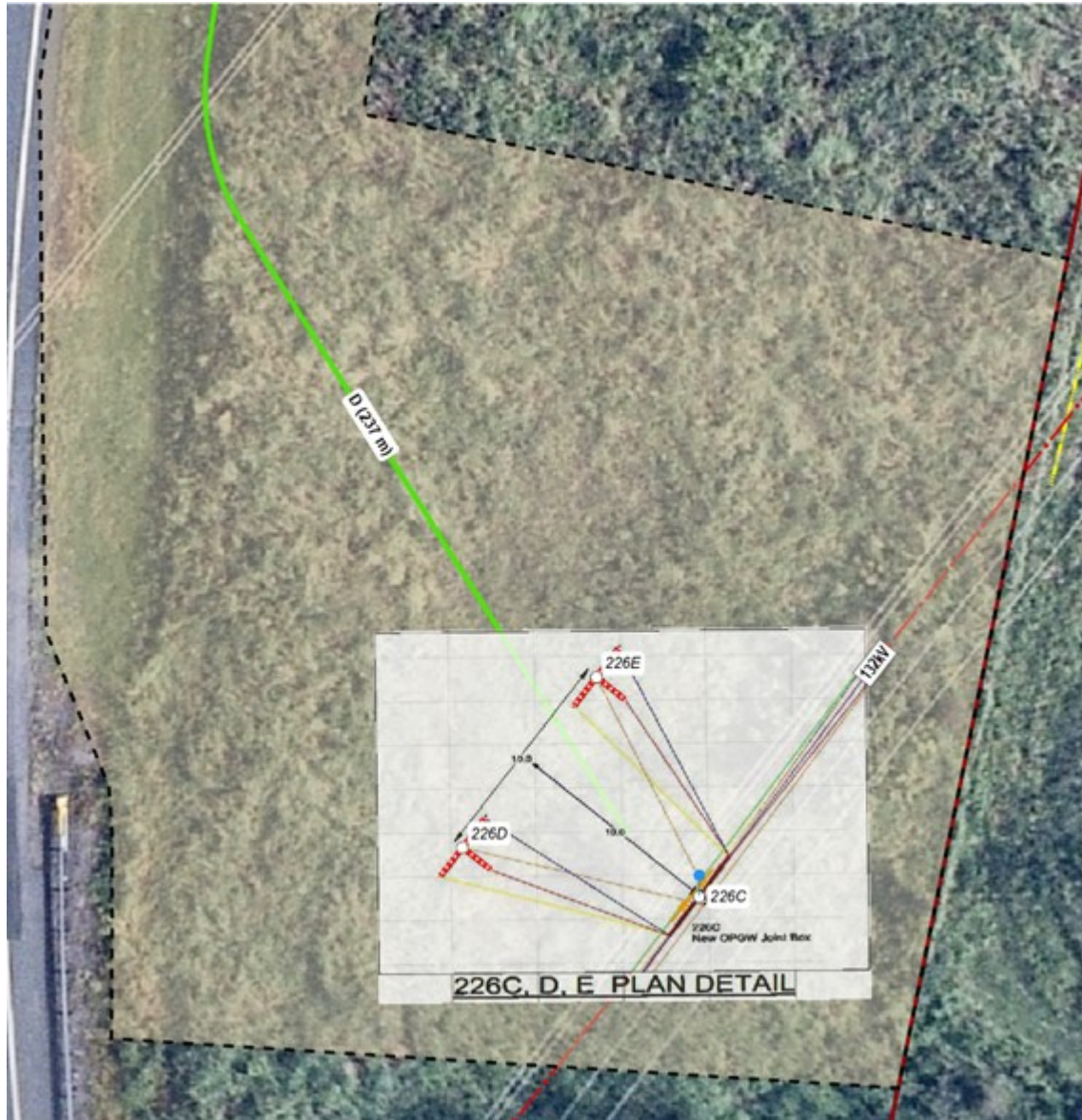
Figure 4.3 Schematic diagram showing proposed cut-in infrastructure to existing 132 kV transmission line in relation to the development footprint
