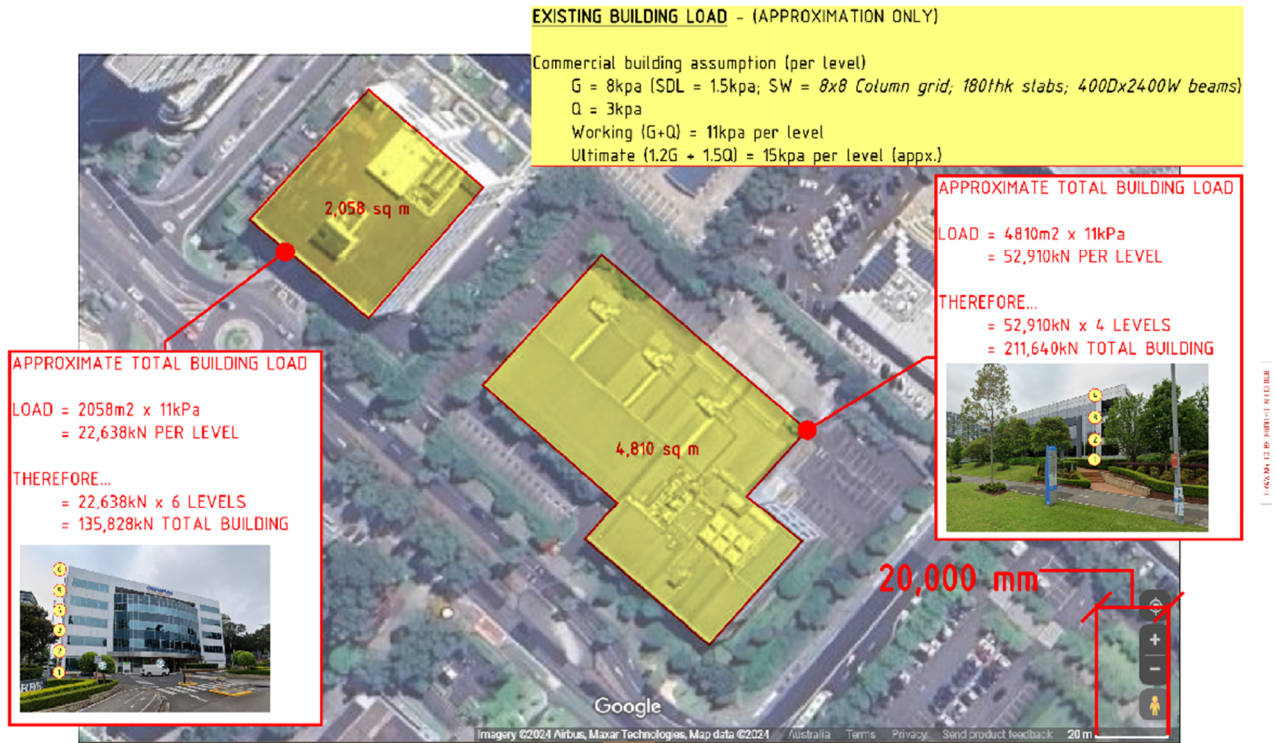
Figure 3: Loads from the Existing Building
