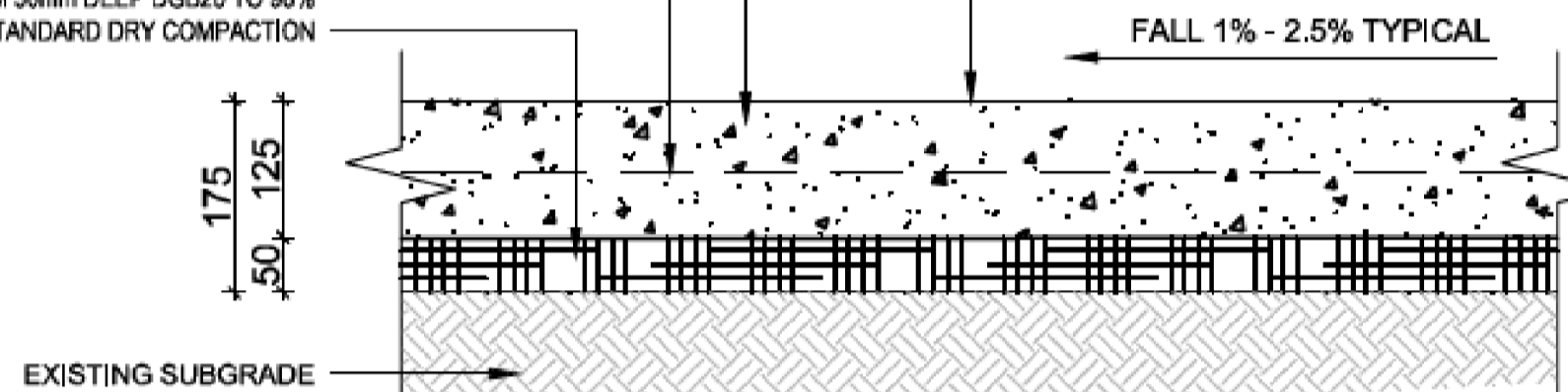
TOWN CENTER PAVEMENT TYPE CONCRETE - TYPICAL COURTESY OF COUNCIL ST DWG PV 1.1
