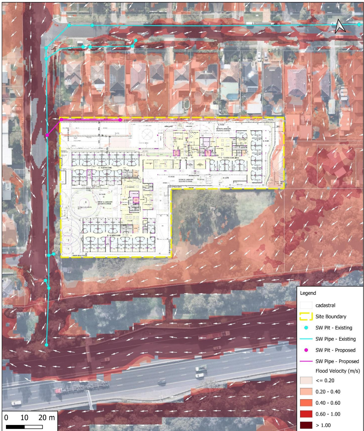
Figure 15 PMF Velocity – Proposed Conditions
