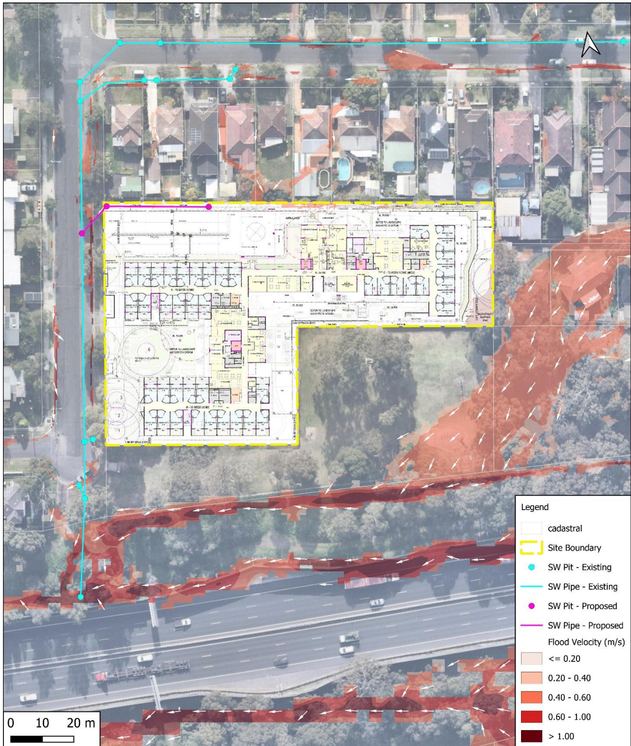
Figure 12 - 1% AEP Overland Flow Velocity – Proposed Conditions
