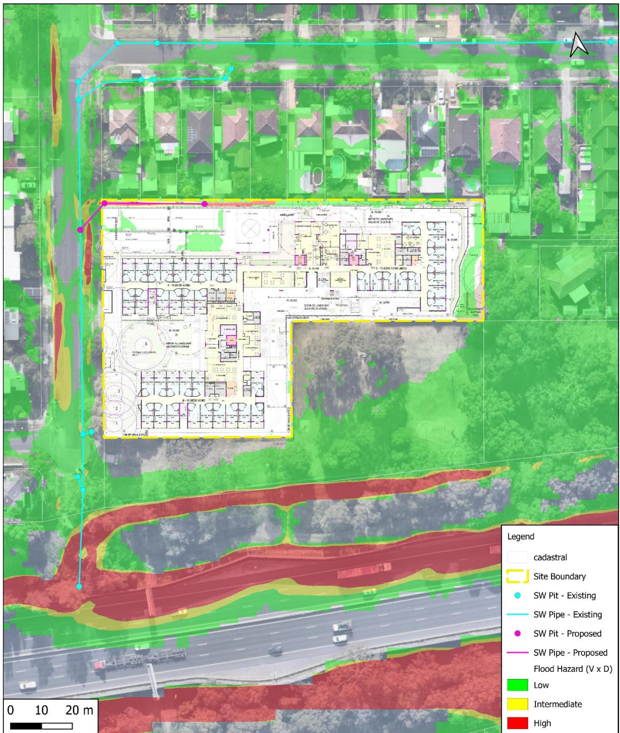
Figure 16 - PMF Hazard – Proposed Conditions
