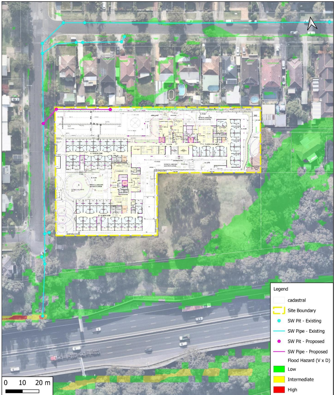
Figure 13 - 1% AEP Overland Flow Hazard – Proposed Conditions
