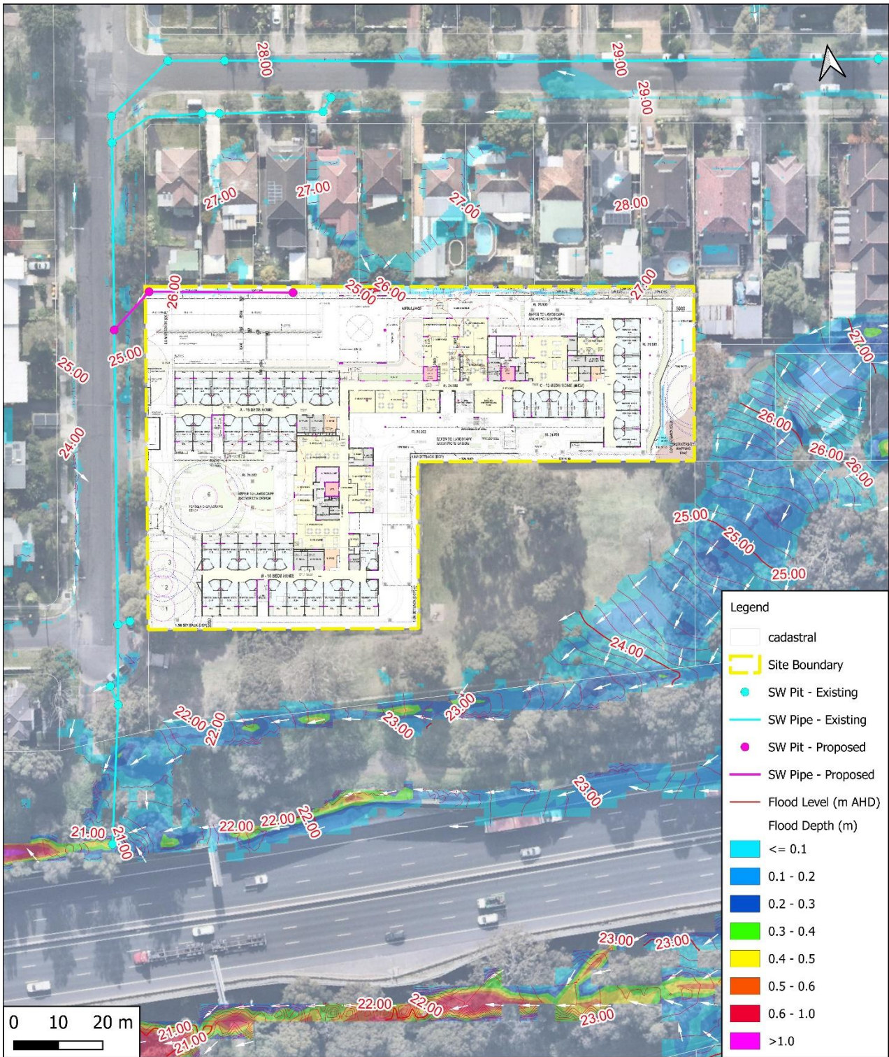
Figure 11 - 1% AEP Overland Flow Level & Depth – Proposed Conditions
