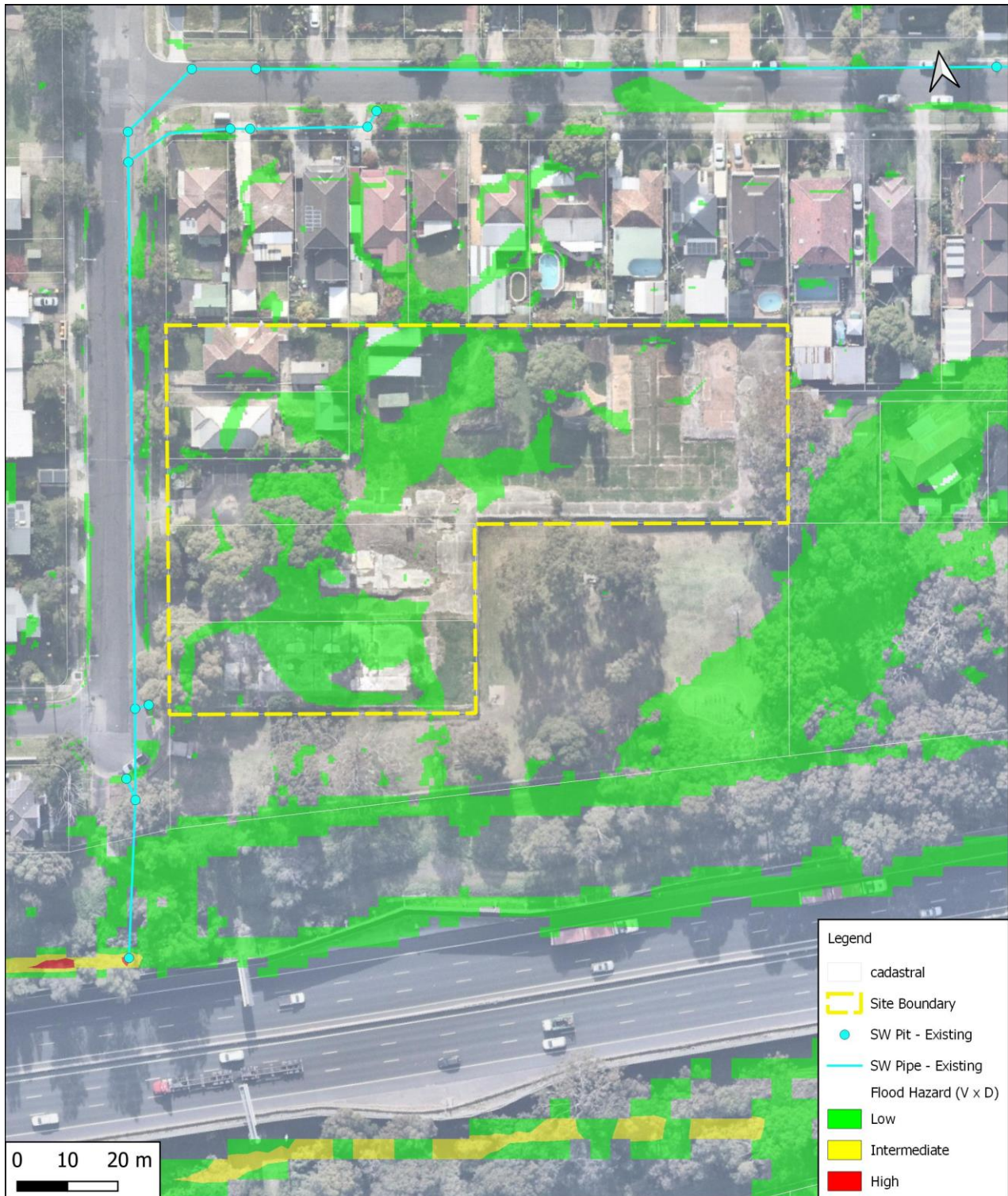
Figure 6 - 1% AEP Overland Flow Hazard – Existing Conditions
