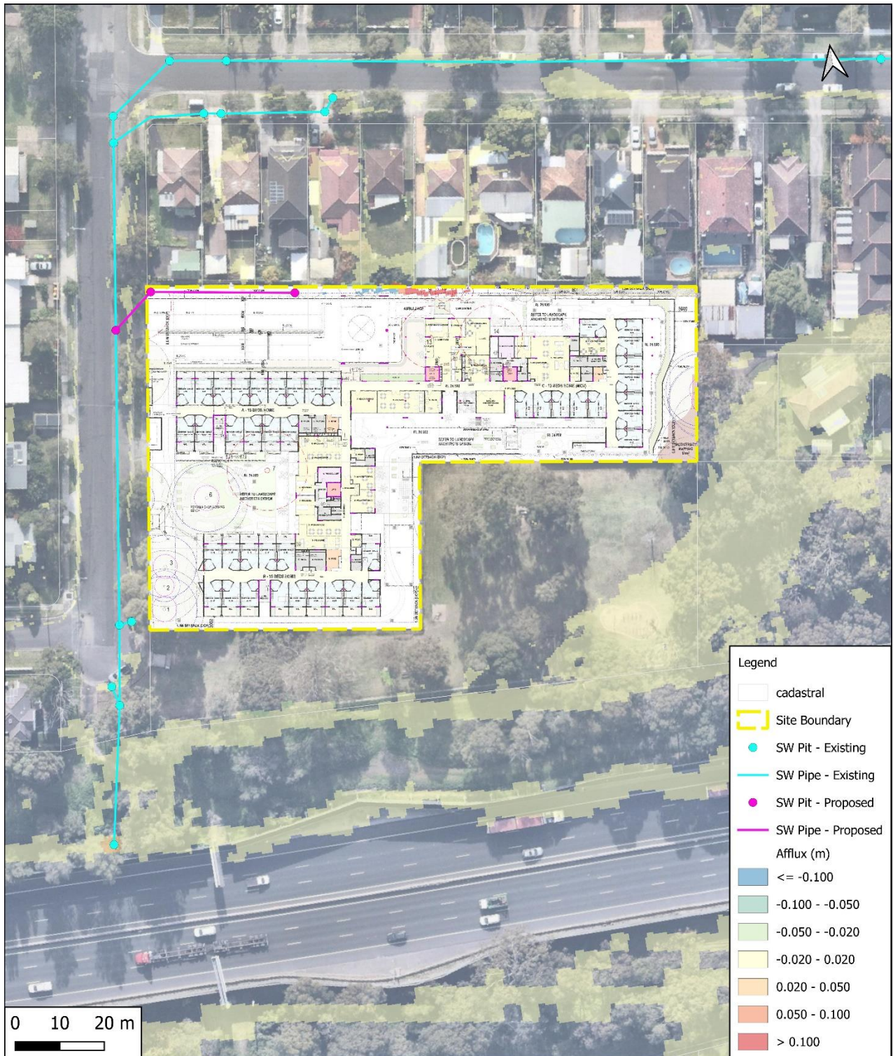
Figure 17 - 1% AEP Flood Level Impacts– Proposed Conditions (Afflux Map)
