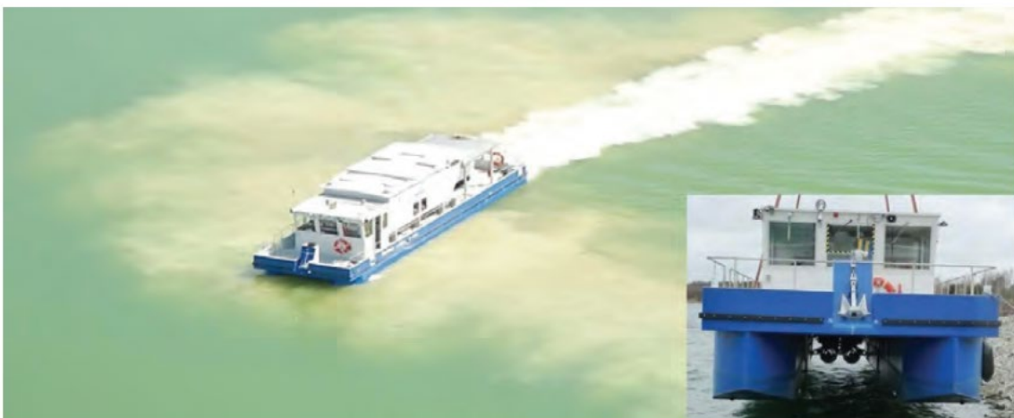
Figure D2: Self-reliant barge/boat application system [Scholz et al., 2007].
