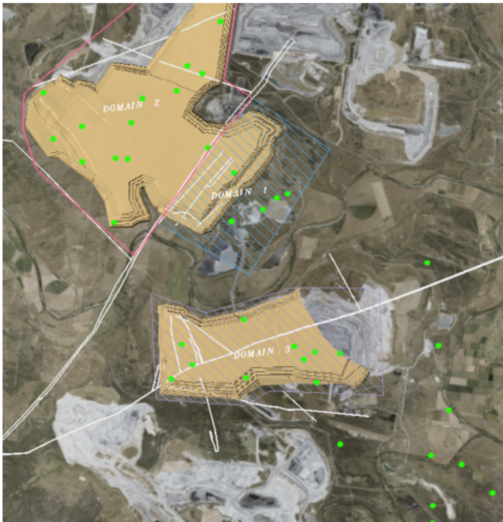
Figure 2: Location of three (3) distinct gas domains at HVO. Green dots represent relevant HVO boreholes used in establishing the model (figure supplied by HVO).
