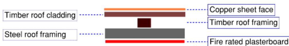
Figure 55 – Existing roof composition breakdown
