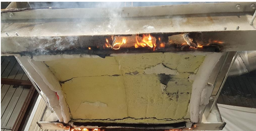
Figure 21 Exposed face of the specimen at the end of the test
