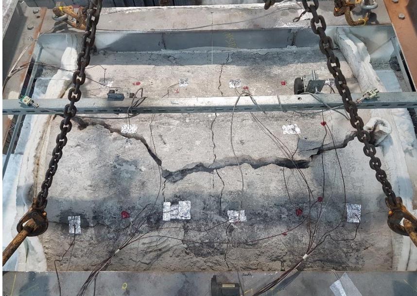
Figure 20 Unexposed face of the specimen at the end of the test
