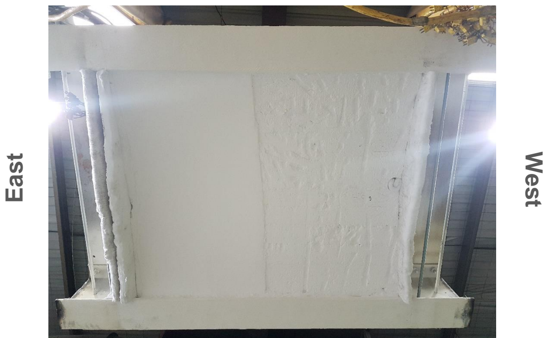
Figure 19 Exposed face of the specimen before the start of the test
