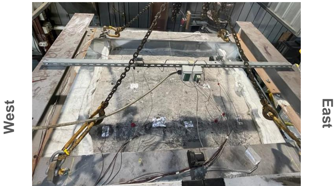
Figure 18 Unexposed face of the specimen before the start of the test
