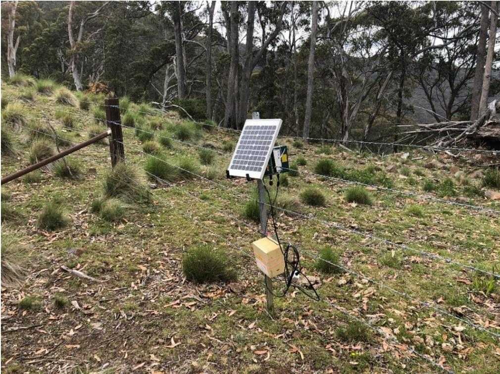
**Photo 7 Ground-deployed acoustic detectors**
