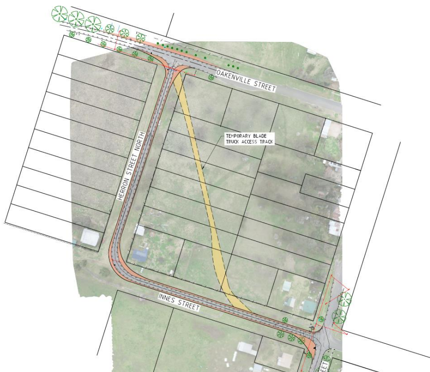
Plate 5 Project design drawings illustrating the areas of additional impact (peach coloured polygons) around Oakenville Street, Herron Street North, Innes Street and Jenkins Street, including the 1 metre width extension on the eastern side of Herron Street North.
