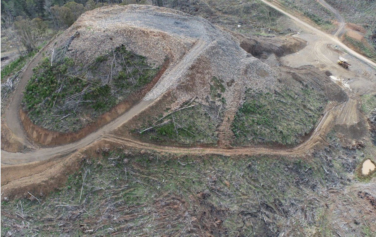
Figure 5 – Oblique aerial view looking north of existing FCNSW quarry operation within proposed Western Operations Area. Note extensive outcrop exposure of columnar-jointed basalt within centre of hill. (GR:327,945 mE 6,519,060 mN – looking N)
