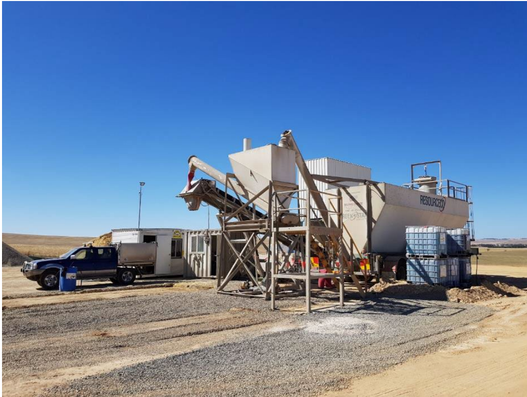
Figure 3-20 Example Concrete Batching Plant – Willogoleche Wind Farm
