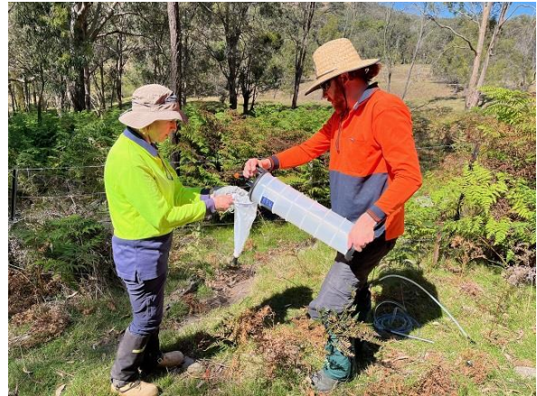
Plate 2: Samples collected using a hand-operated bilge pump were filtered through the stygofauna net and then emptied into a labelled sample bottle.
