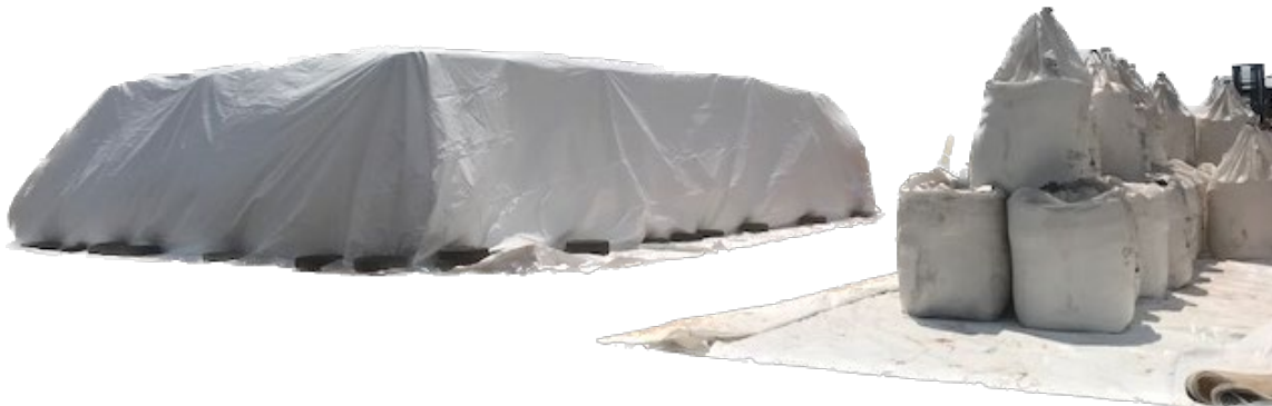
Figure 1. Illustration of the liners proposed to encompass the bagged AN.
