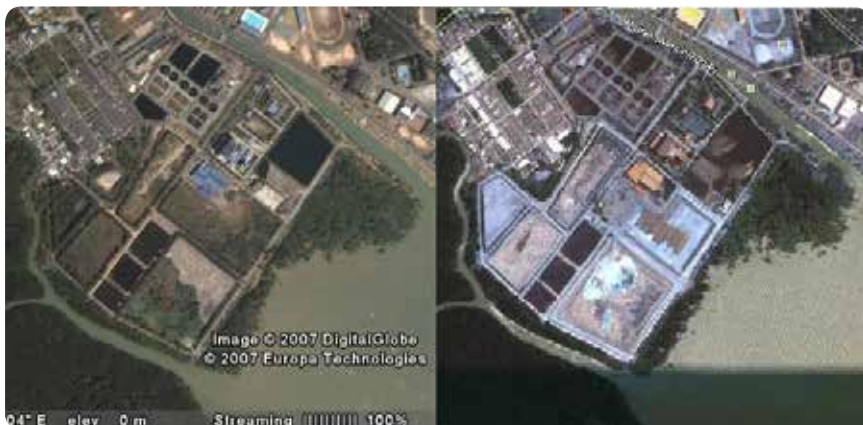
Figure 17: From the comparison between the photomap from 2007 (left side) and 2010 (right side), it is clear that land use has changed around the waste incinerator in Phuket. The large grey area at the south-east edge of the incinerator was an area with fly ash dumping in 2007. Source: Petrlik (2011).
