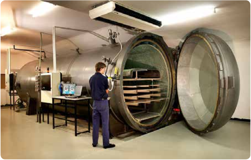
Figure 32: Example of a steam autoclave for medical waste. Source: United Medical Industries
