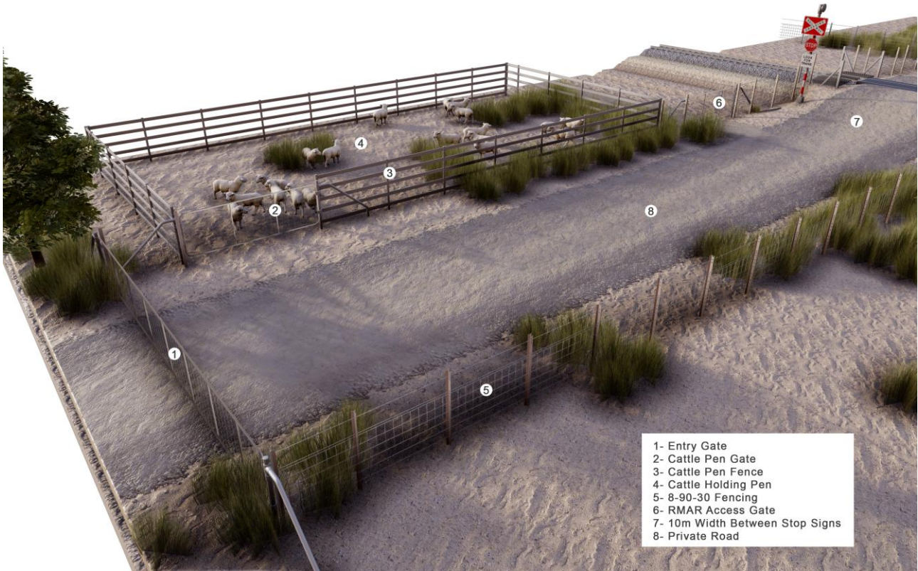
FIGURE 7-2 INDICATIVE LAYOUT OF A PRIVATE STOCK CROSSING STOCK HOLDING PEN (SUBJECT TO DETAILED DESIGN)
