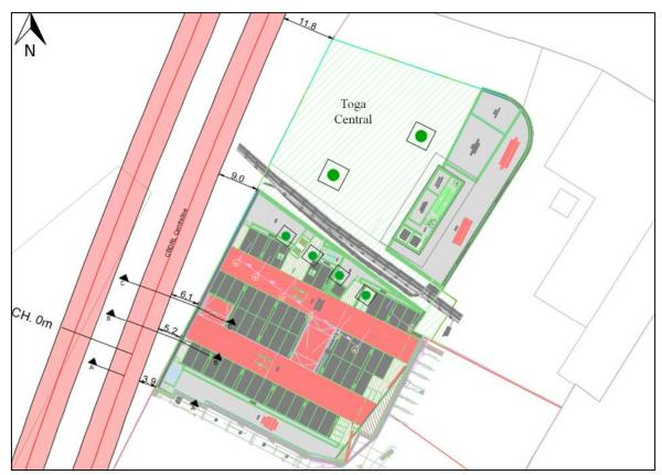
Figure 6-3: Plan view illustrating horizontal distances from the CBDRL tunnels to proposed development (source: project rail interface report [2])
