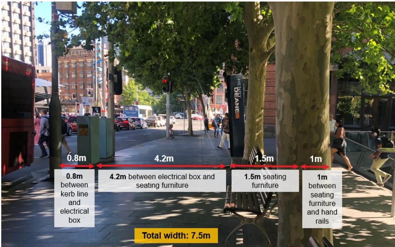
Figure 10: Existing Footpath Measurements (Segment 3: Lee Street Footpath, adjacent HDP staircase)
