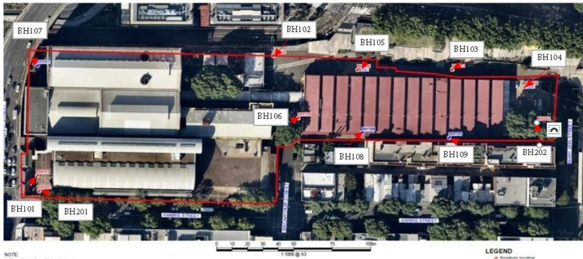
Figure 4-16: Location of geotechnical boreholes associated with the study area. Harris Street runs horizontally along the bottom of the image and Mary Ann Street runs vertically at the right-hand side of the image (Source: Douglas and Partners)
