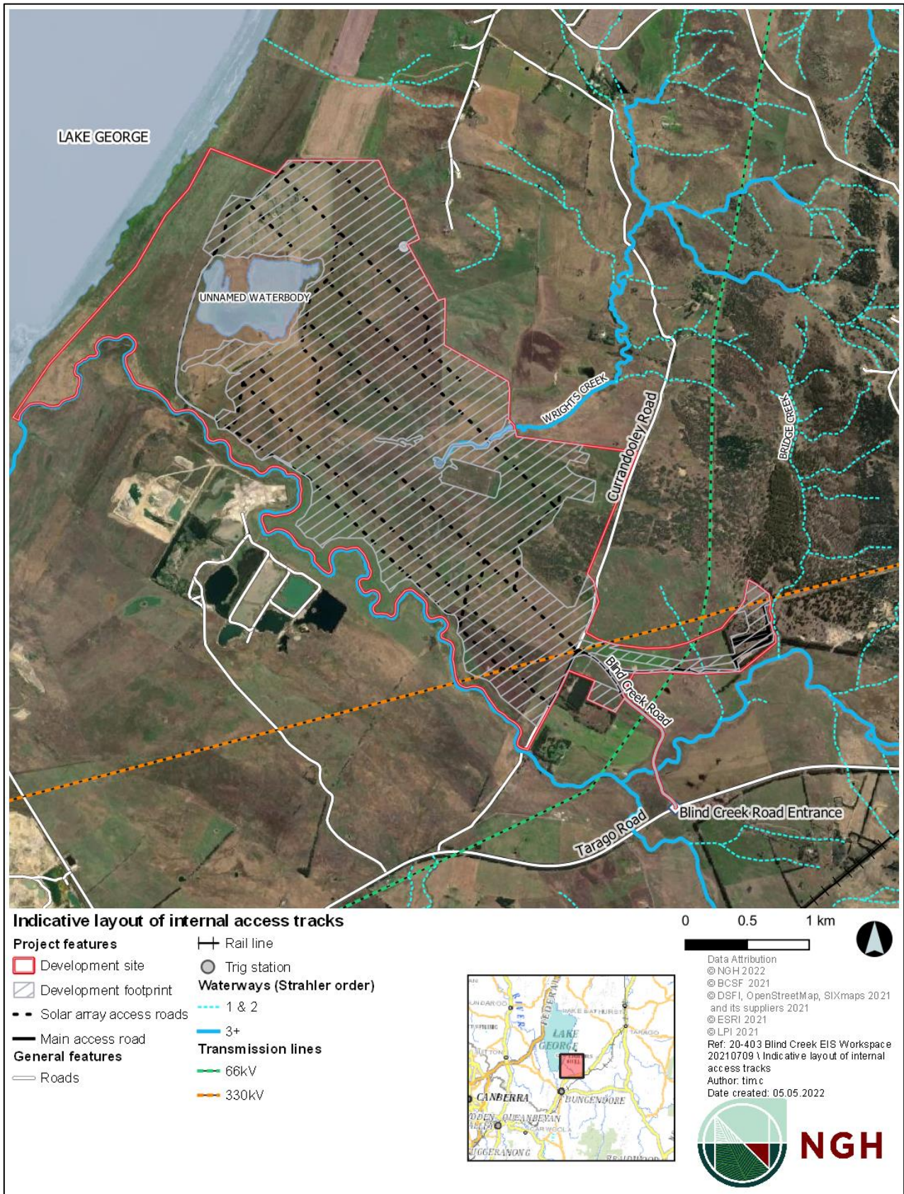
Figure 1-13 Indicative layout of internal access tracks
