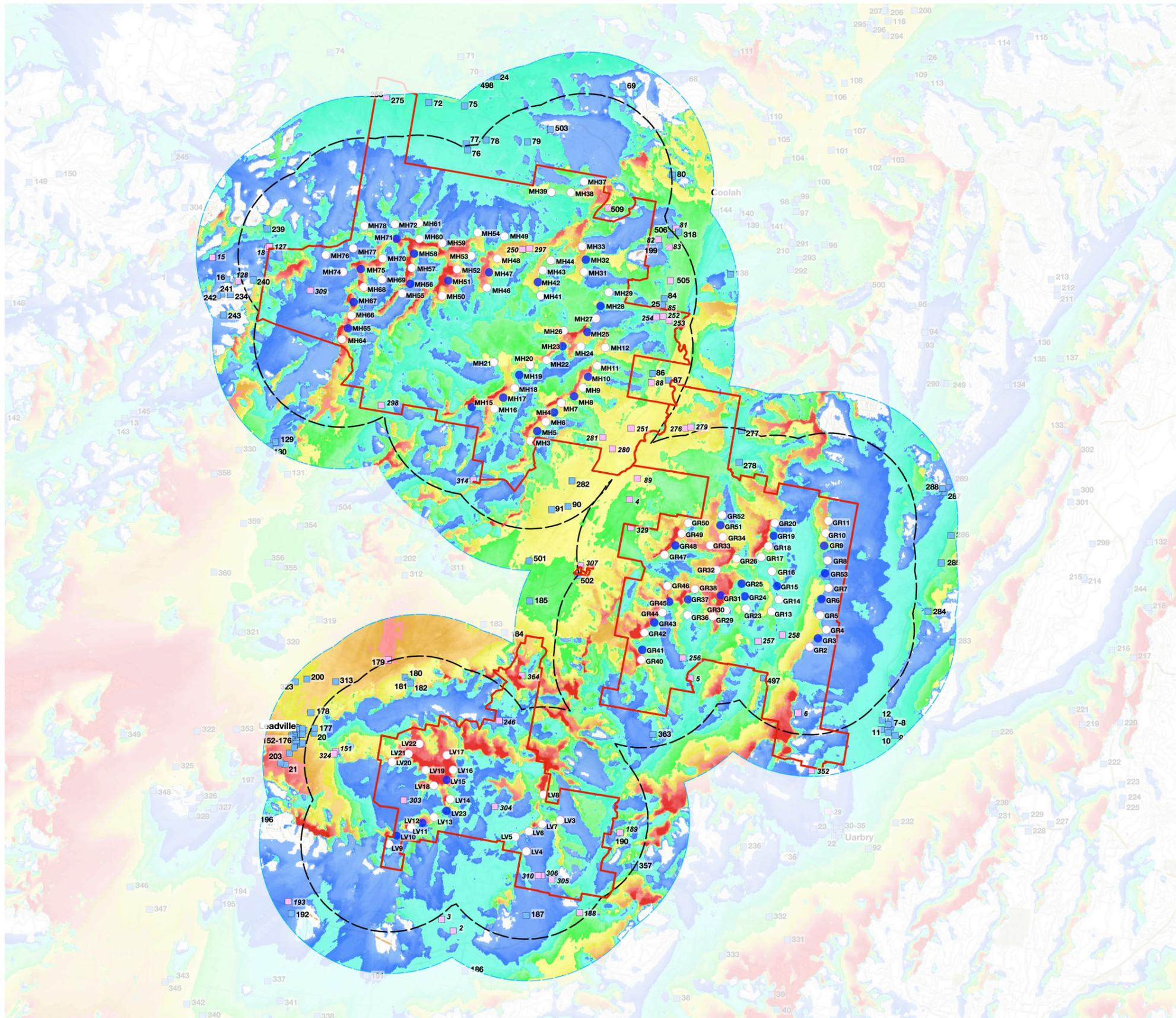
**Figure 12. Theoretical Visibility of Turbine Aviation Hazard Lighting**
