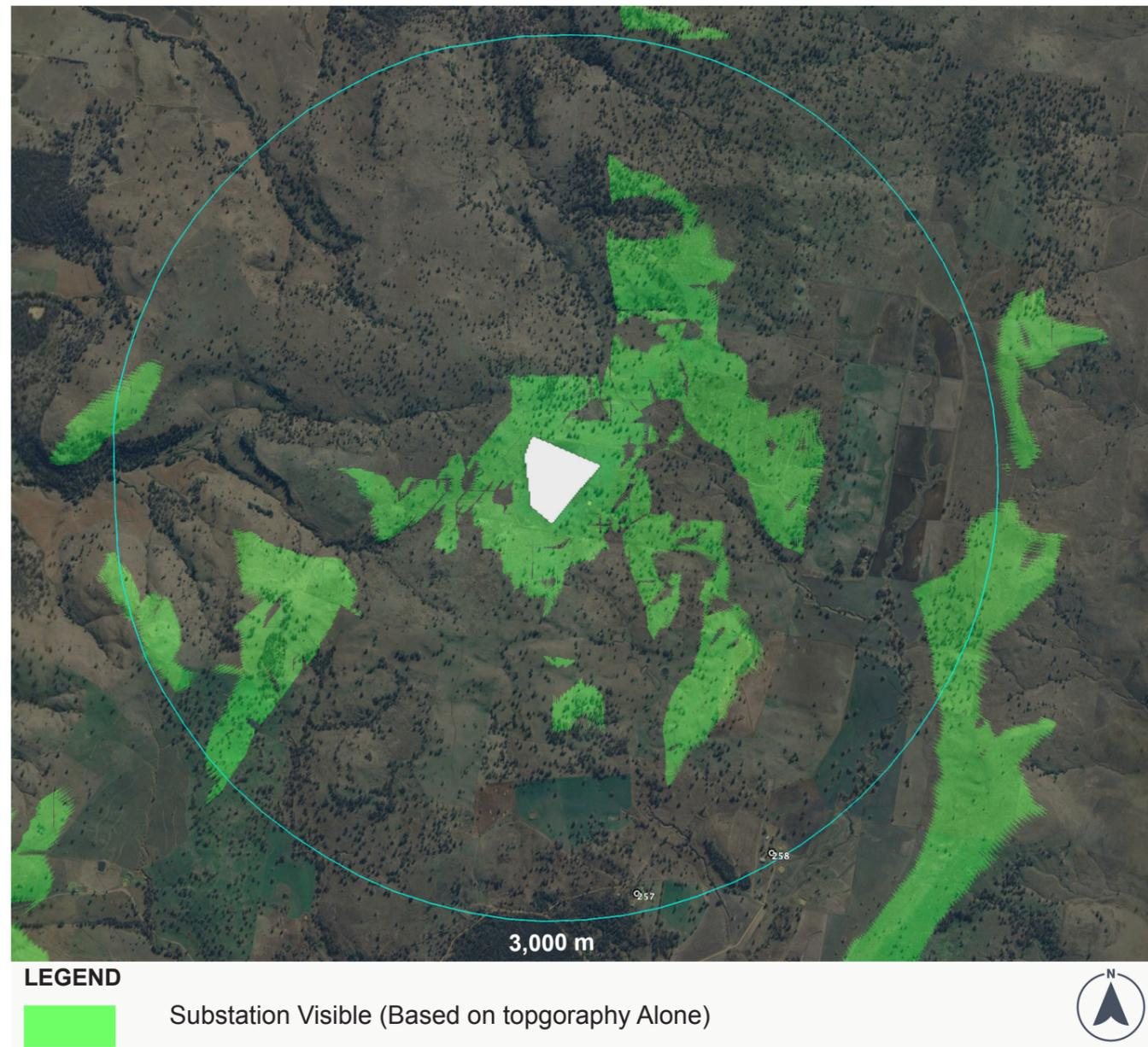
**Figure 18. ZVI - Girragulang Road (GR) Substation**
