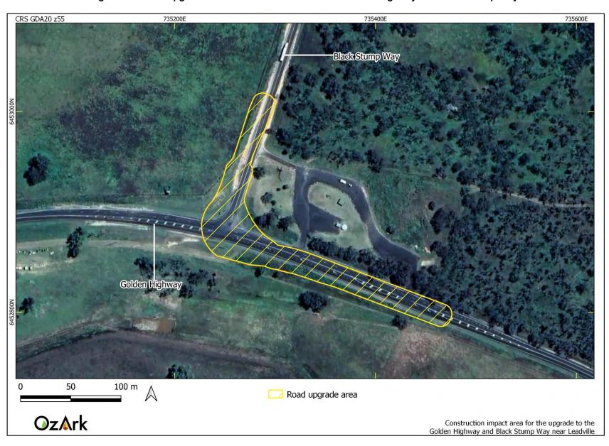
Figure 1-5: Road upgrade area at the intersection of the Golden Highway and Black Stump Way.
