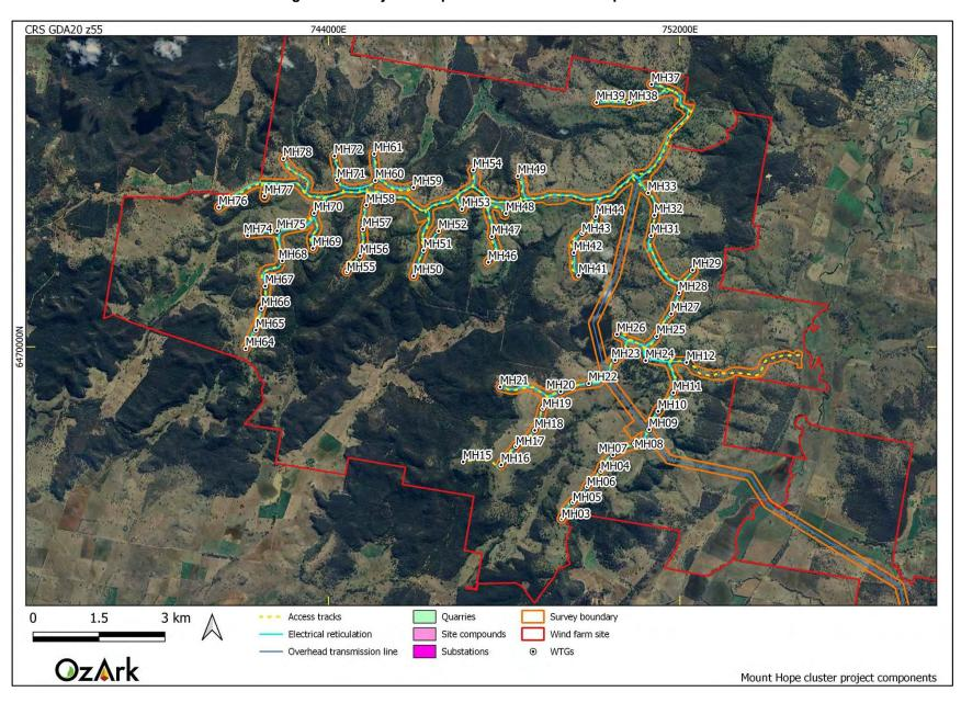
Figure 1-2: Project components at the Mount Hope cluster.
