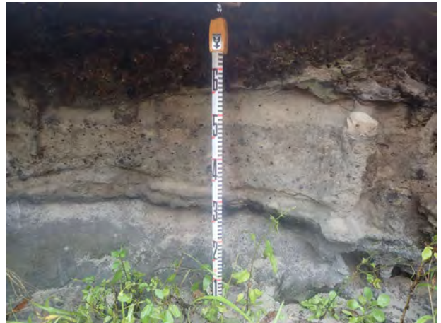
Figure 17 – Sectional view of fill below concrete slab near Bunnerong Stormwater Channel
