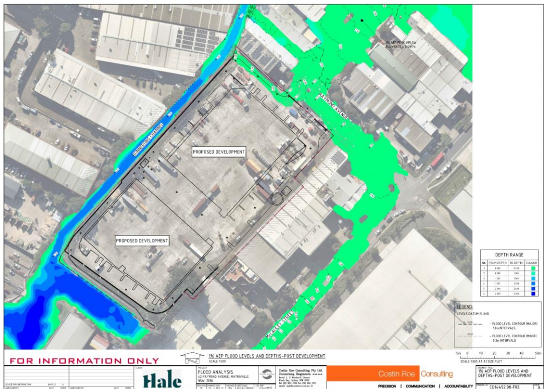
Figure 7.10: 1% AEP Post-developed Level and Depth Output
