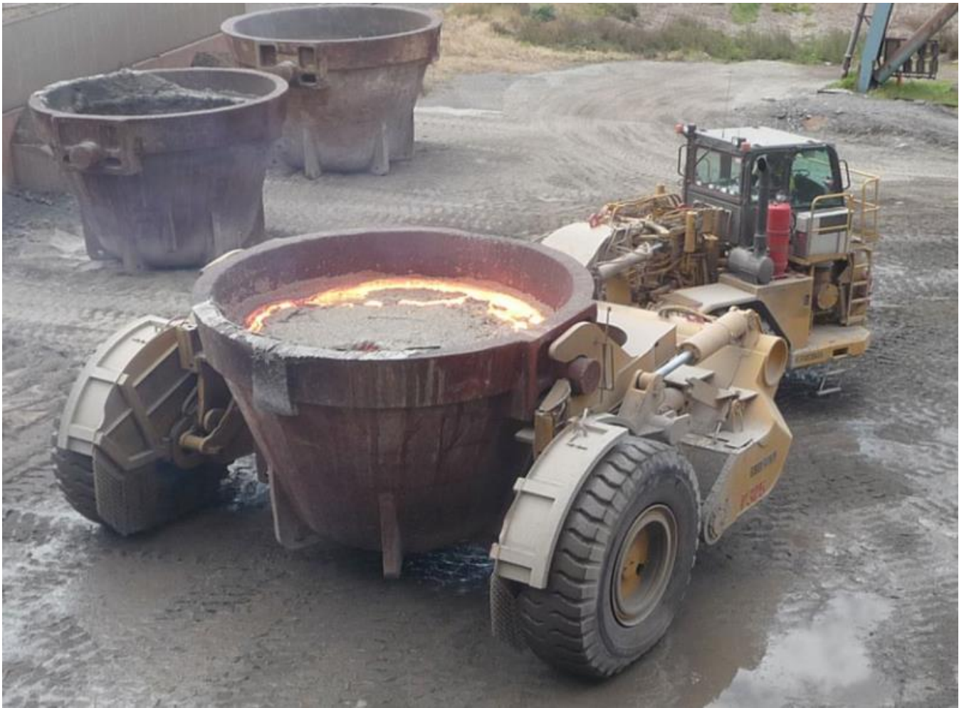
Figure 5.5 Slag pot Kress carrier in operation during previous 6BF campaign
