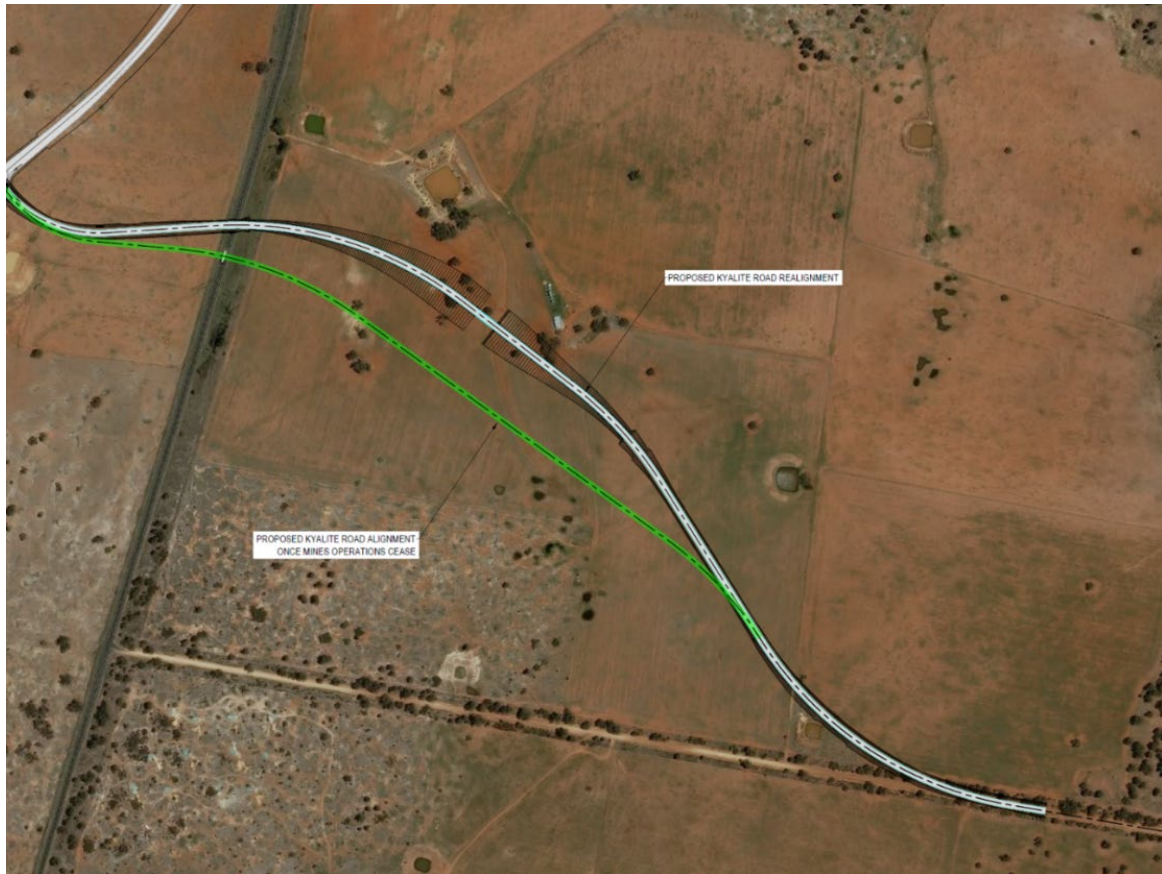
Figure 7 – Proposed Kyalite Road Realignment after the Completion of the Mining Operation
