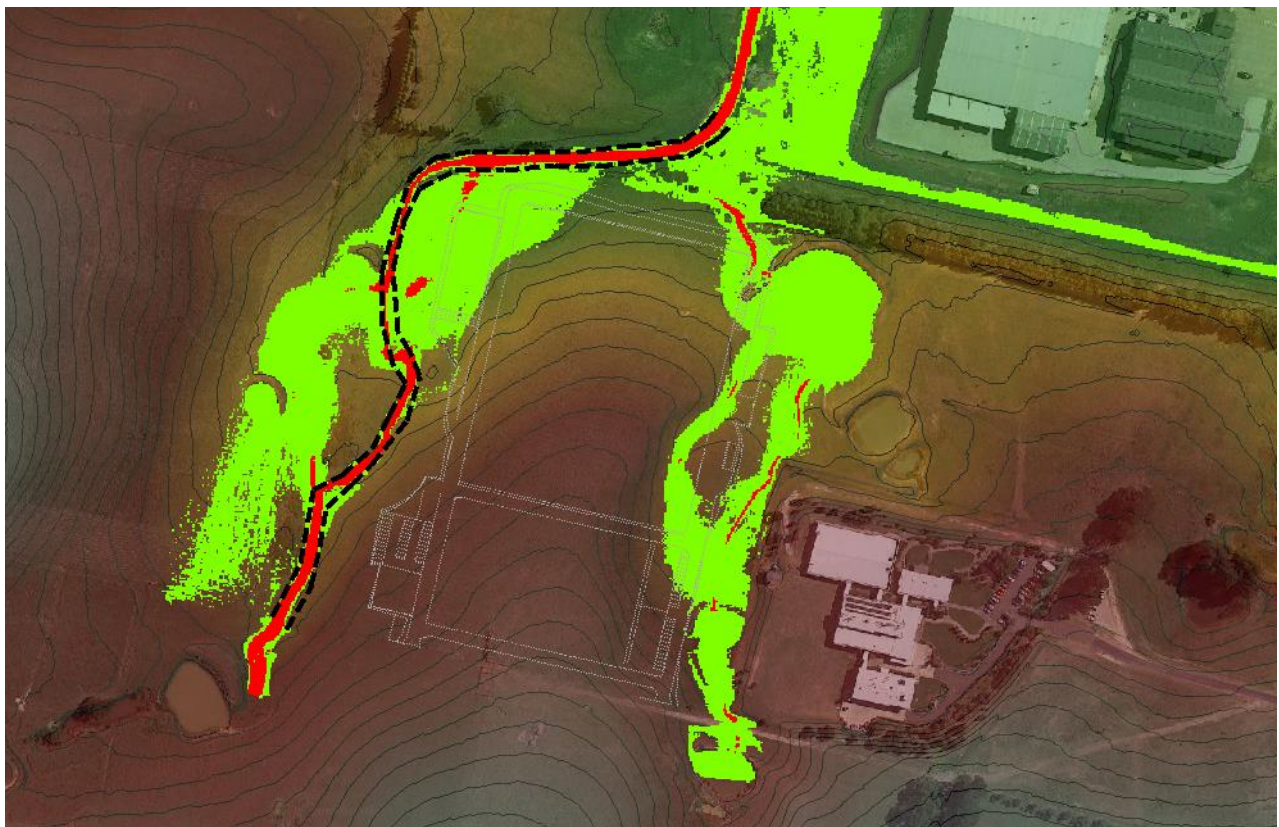
Figure 1 Estimated Floodway overlain on existing 1 in 100 AEP Depth Velocity map, where green is DV < 0.25 \text{ m}^2/\text{s}
