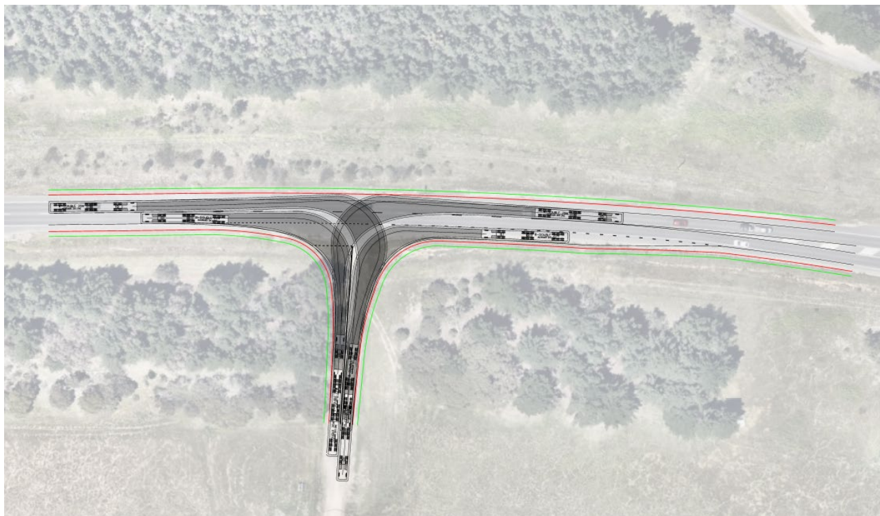
Figure 4-13 Proposed intersection layout and swept paths following sensitivity analysis
