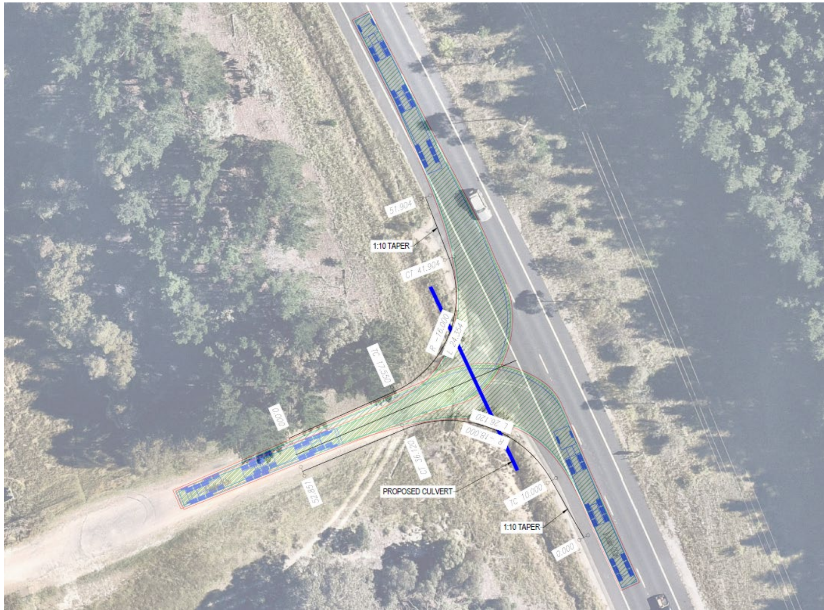
Figure 4-3 B-Double Vehicle Swept Path
