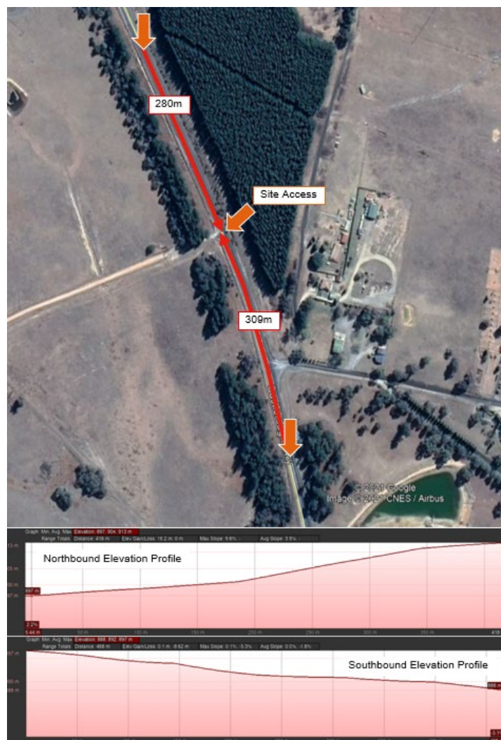
Figure 4-6 Access sight distances and longitudinal grades
