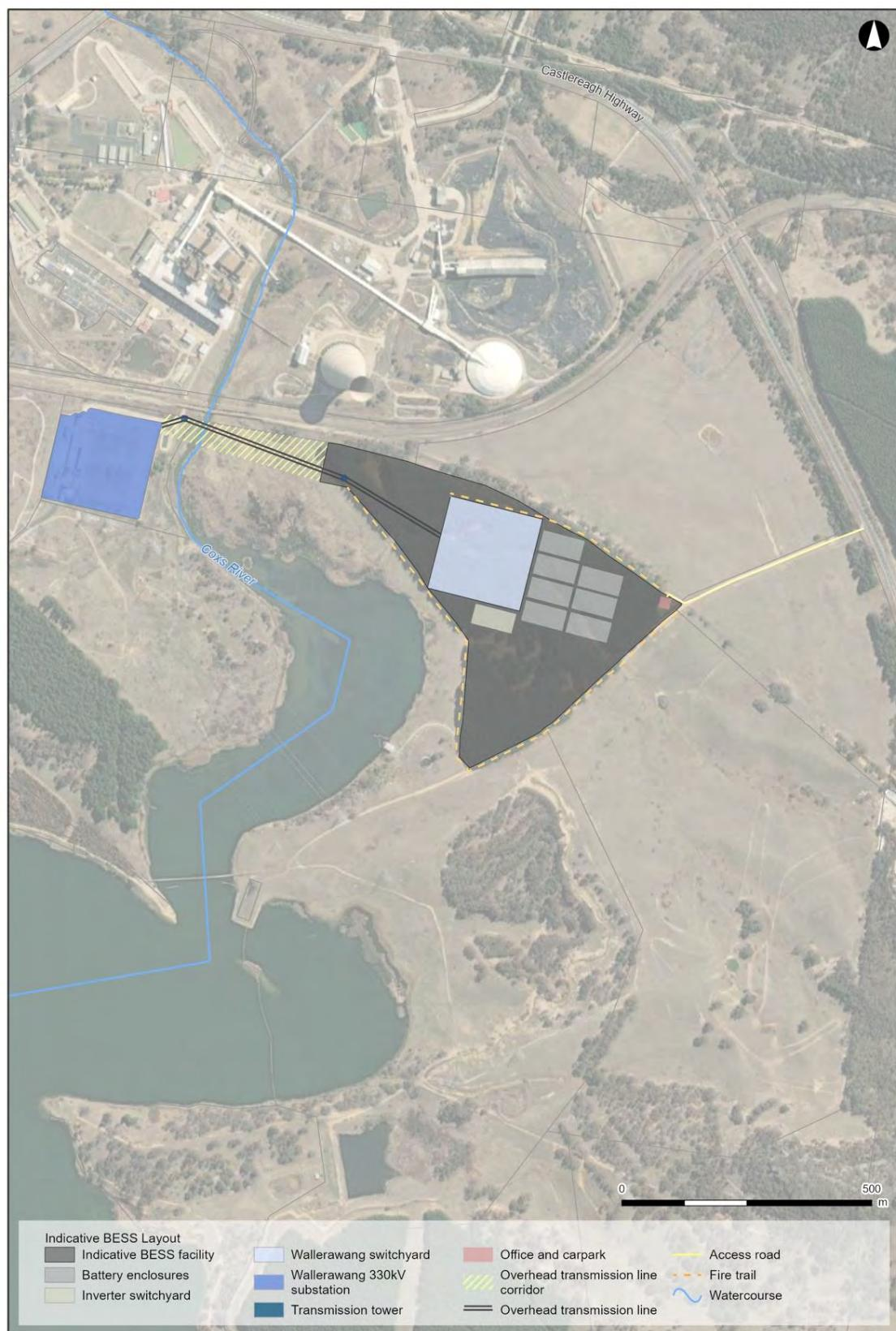
**Figure 1 Proposed EIS site layout for Wallerawang Battery Energy Storage System**
