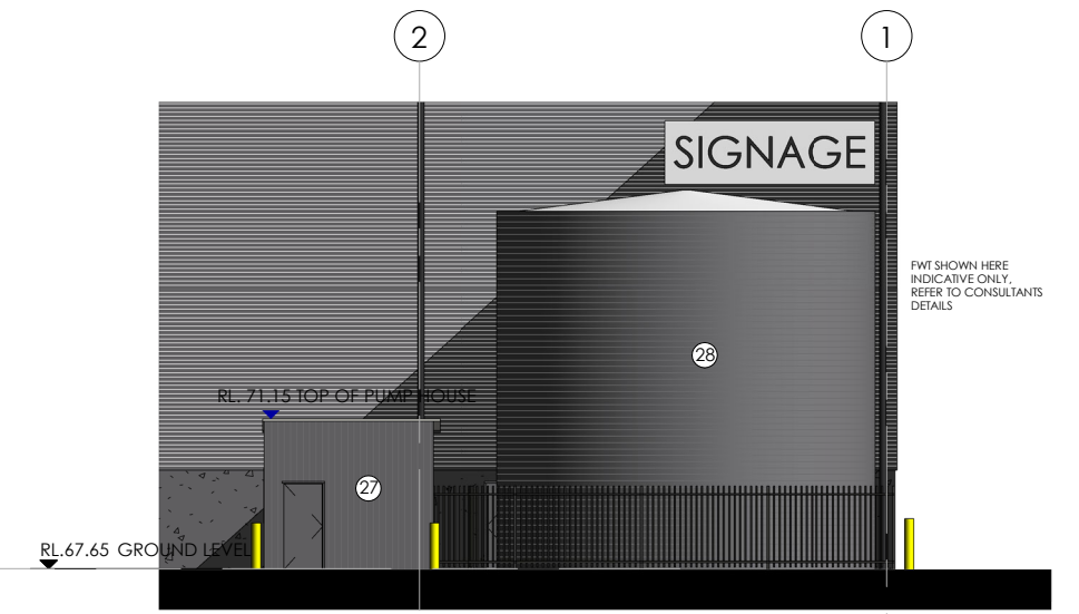
10 PUMP HOUSE ELEVATION - TYP 1 : 200
