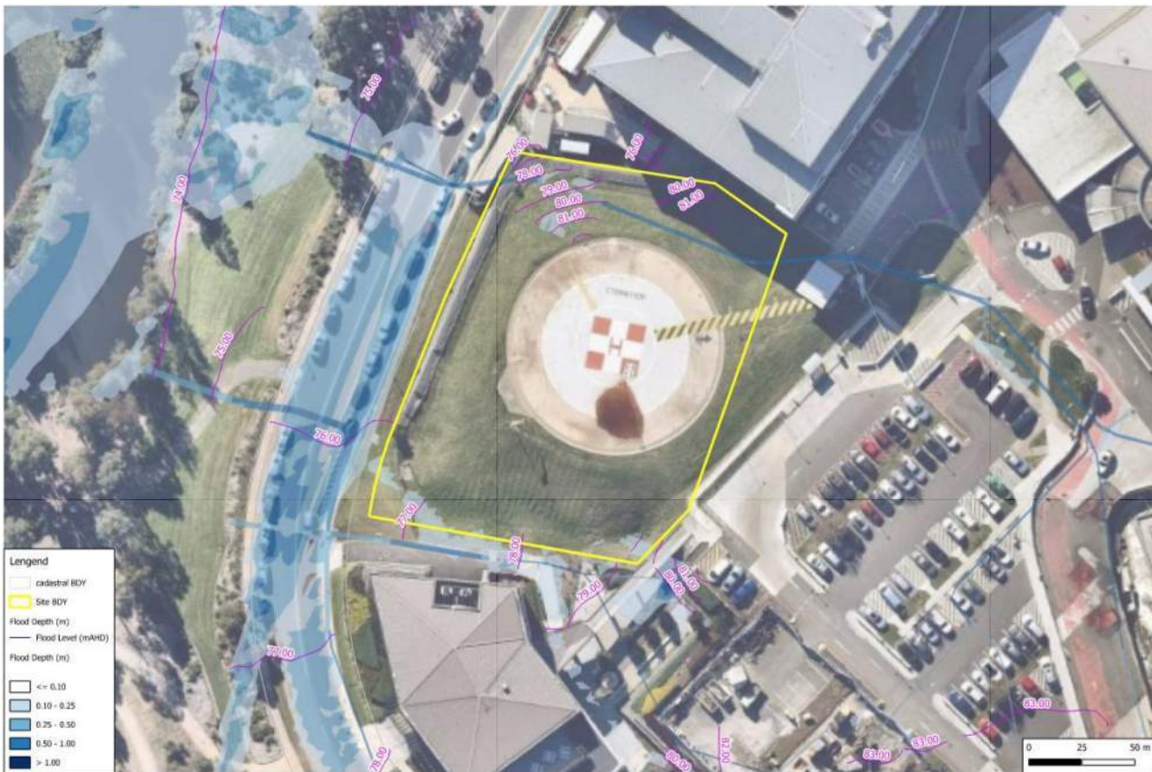
Figure 5 - Received flood Results (CSS) - 1% AEP Flood Event
