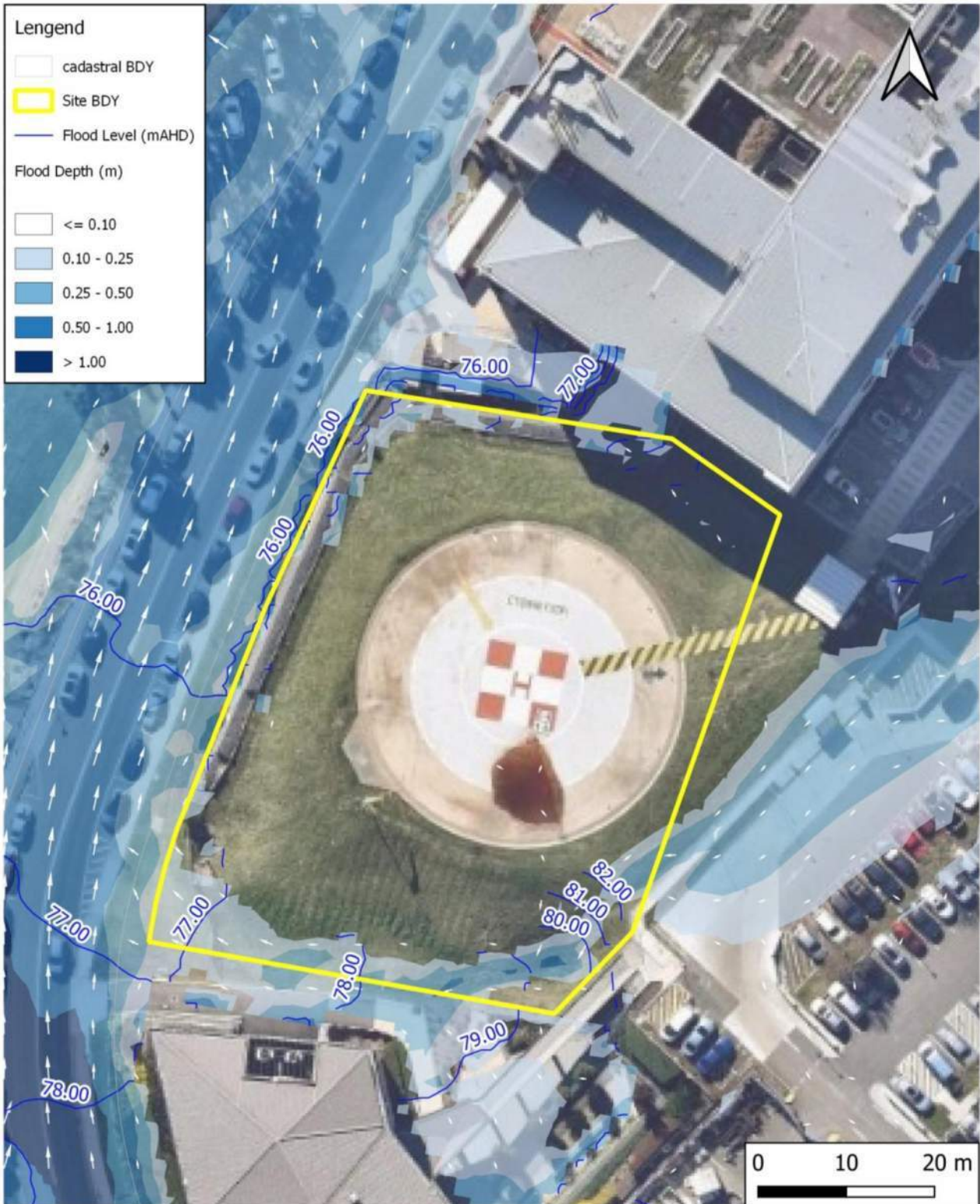
Figure 11 - Flood Levels & Depths (PMF) – Existing Conditions
