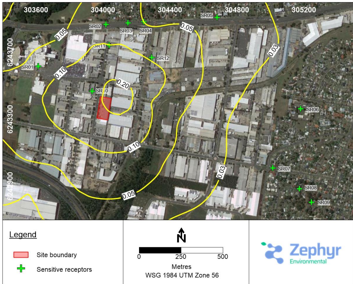
Figure 7-2: Predicted maximum 24-hour average PM 2.5 concentrations due to the proposed WTF (µg/m 3 )
