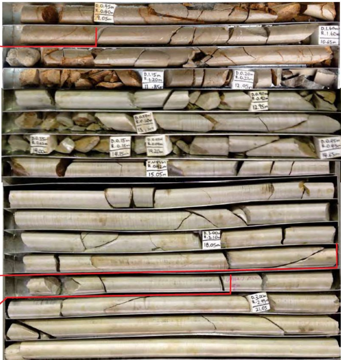
Figure 4.2: Rhyolite intrusive rock, showing limited fracturing below the surface zone and minimal iron staining
