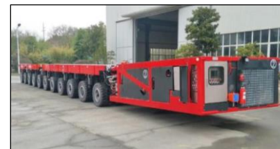
Self-propelled modular transporter (SPMT)
