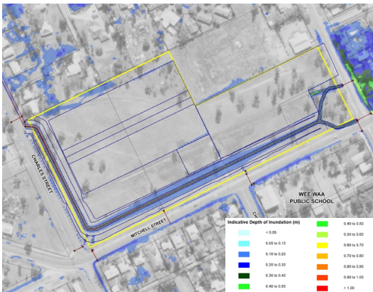
FLOOD INUNDATION LEVELS – WITH RECOMMENDATIONS 20% AEP (5 YEAR EVENT)
