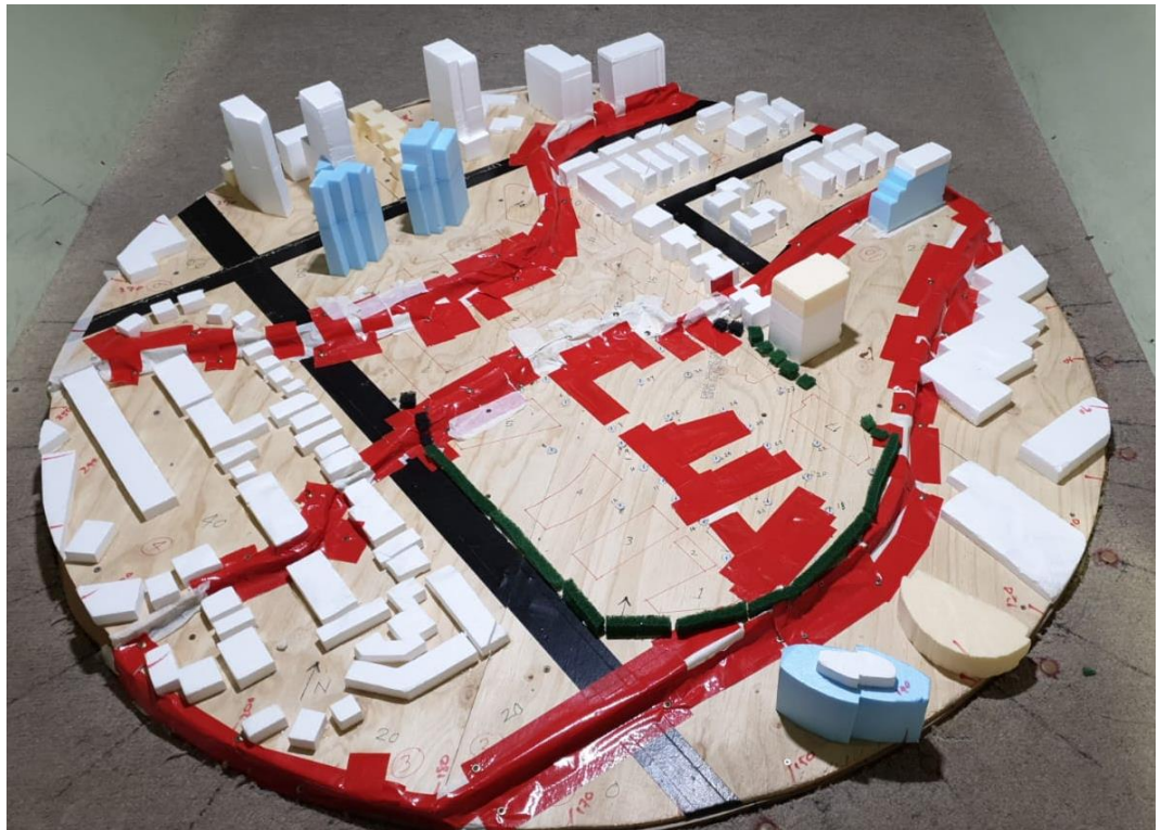
Figure 9 1:400 Scale Proximity Model in Wind Tunnel
