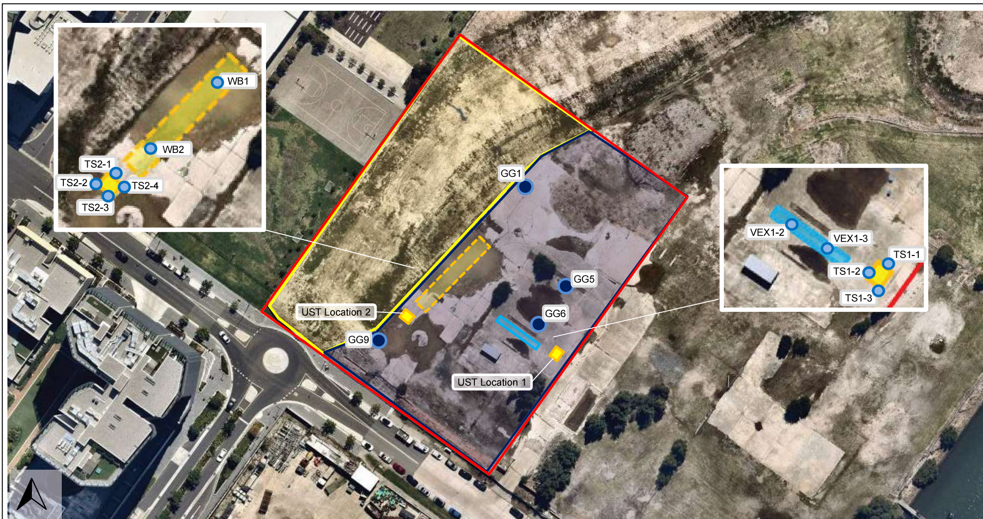
Figure 4: Site Layout Plan – Locations of USTs and Other Infrastructure
