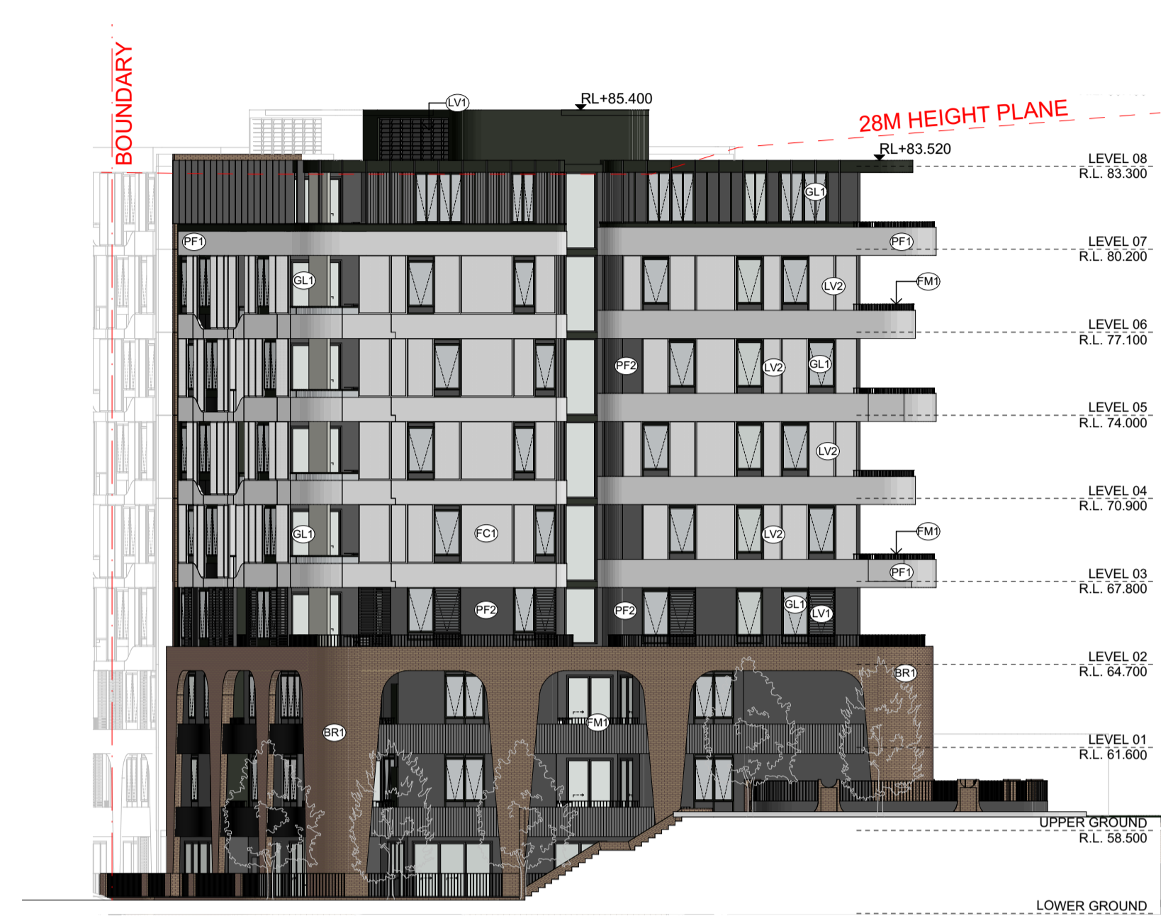
ES BLDG. E SOUTH ELEVATION SCALE: 1:200@A1
