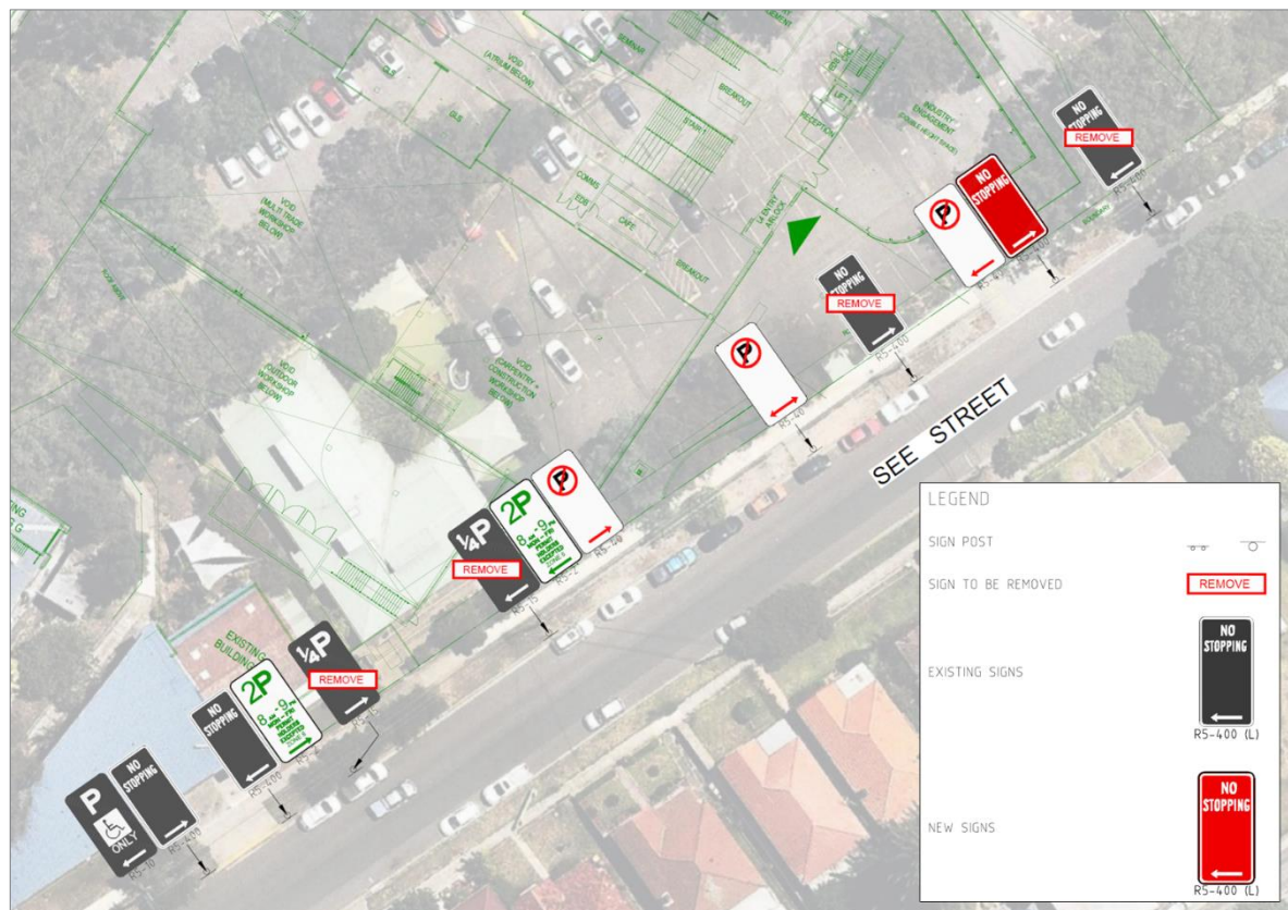
Figure 1: Indicative plan of kerbside restrictions along See Street frontage of the multi-trades and digital technology hub
