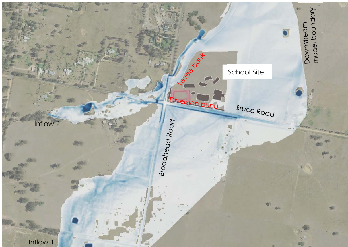
Figure 4: Post development site with levee bank protection along Broadhead and Bruce Road.
