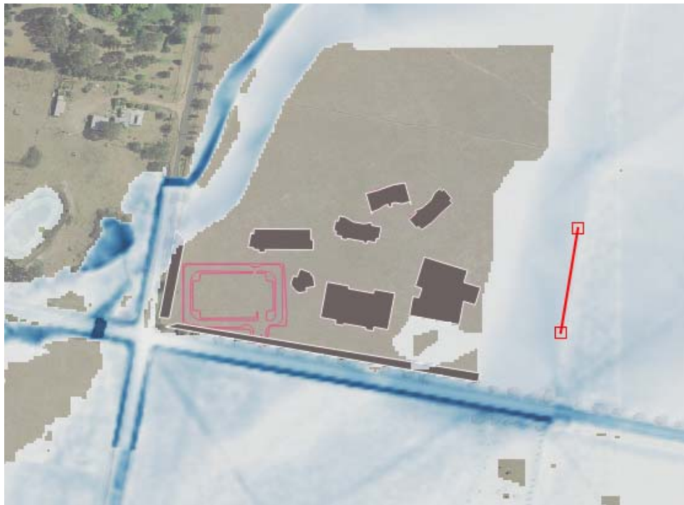
Figure 5: Section taken along adjacent boundary to check flow depths and velocities (shown in red).
