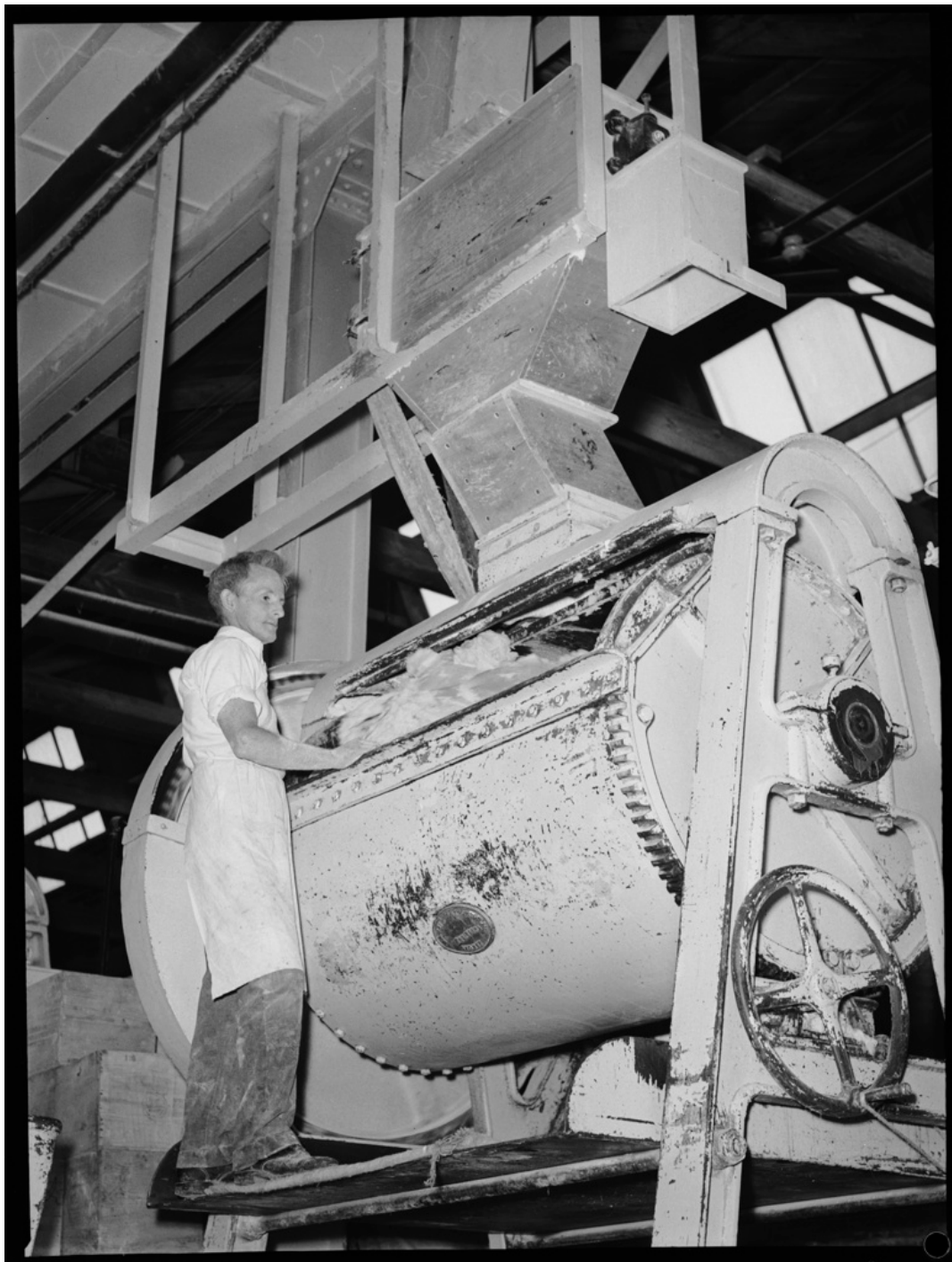
Figure 172. A male Arnott's employee operates a machine used for kneading biscuit dough. Olson, 1938. Source: SLNSW ON 388/Box 031/Item 100.
