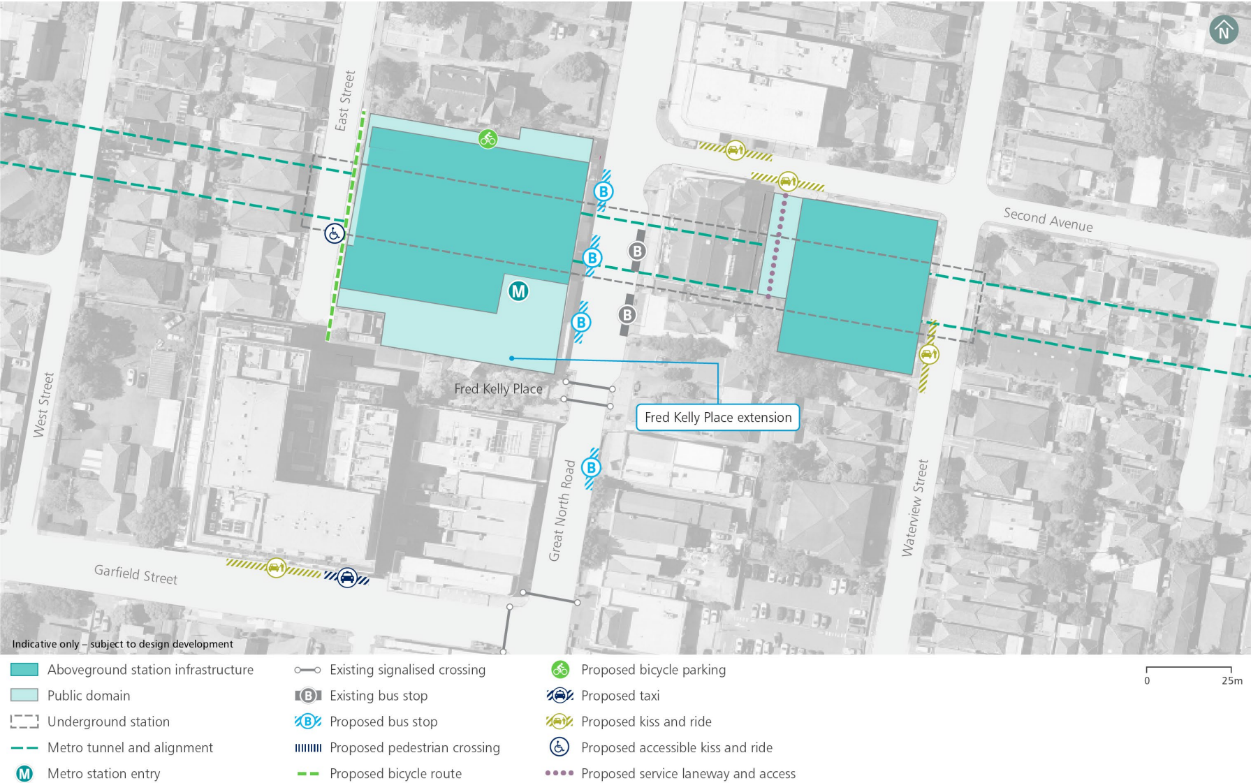
Figure 8-1 Indicative layout and key design elements – Five Dock Station
