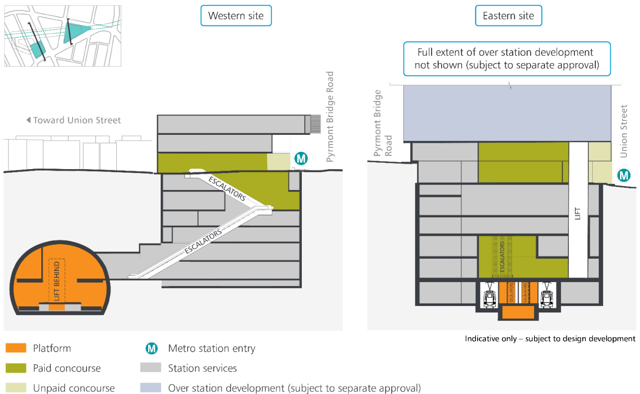
Figure 10-3 Indicative cross-sections – Pyrmont Station
