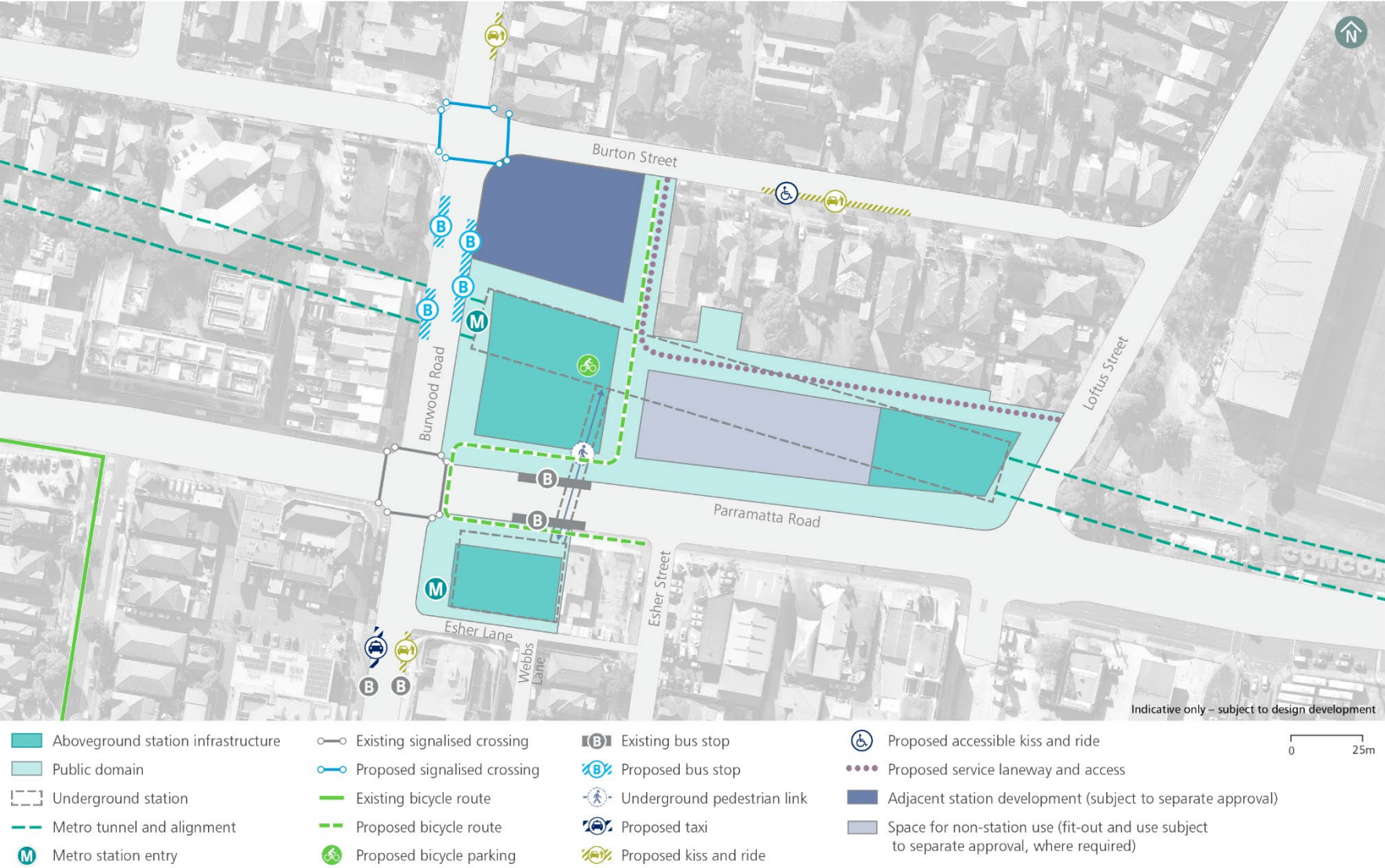
Figure 7-1 Indicative layout and key design elements – Burwood North Station
