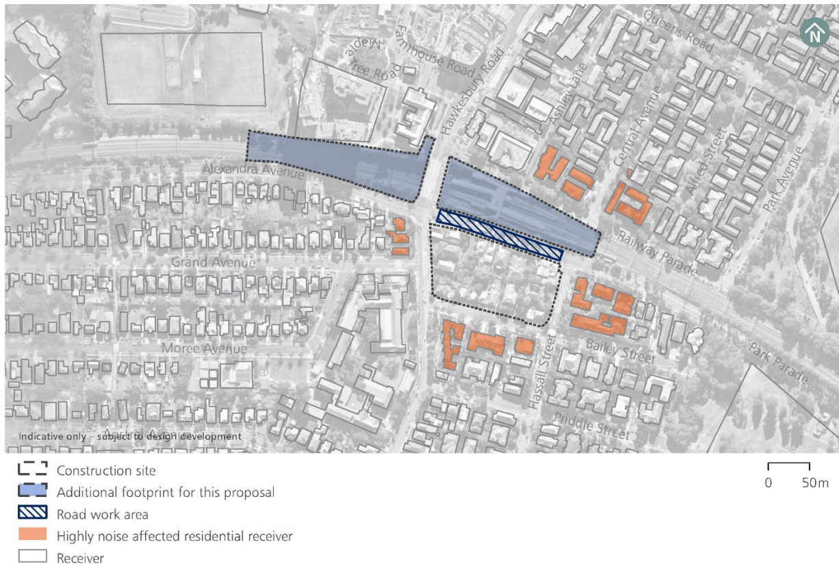
Figure 2-4 Highly noise affected residential receivers resulting from proposed refinements – Westmead metro station
