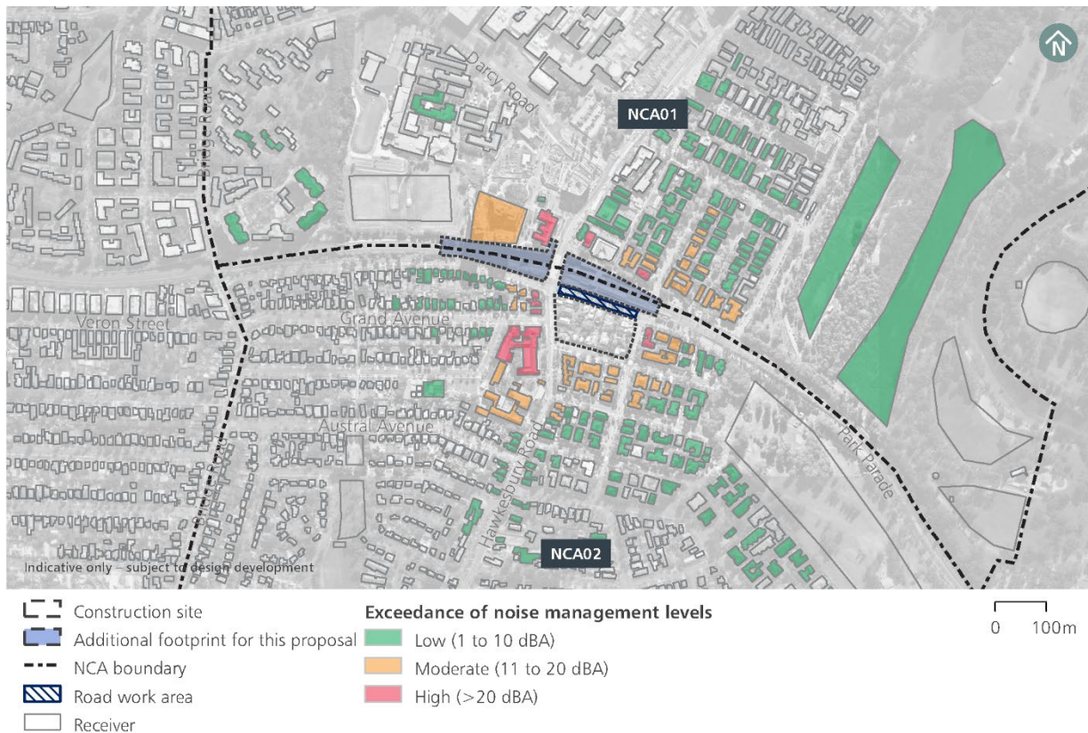
Figure 2-3 Worst case daytime airborne noise ('peak' road work) resulting from proposed refinements - Westmead metro station
