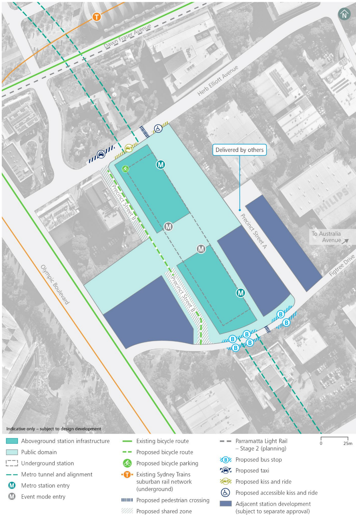
Figure 2-21 Exhibited indicative site layout and key design elements – Sydney Olympic Park metro station (Figure 9-1 of the Environmental Impact Statement)
